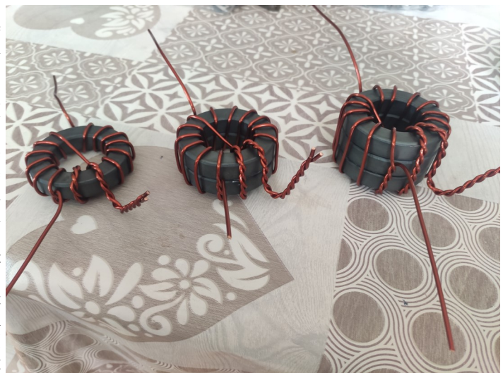
1 Toroid for up to 100W, 2 Toroids for > 100 W and 3 Toroids for 500W - 1 KW
