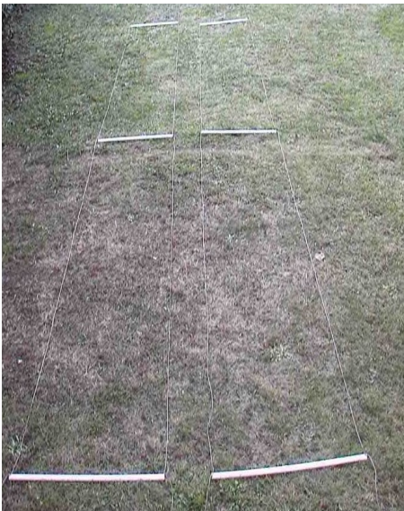
Spreader attached to the wires of each leg of the antenna
