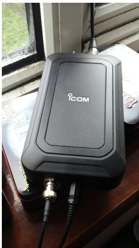
The AH-705 Auto Tuner powered by internal batteries
