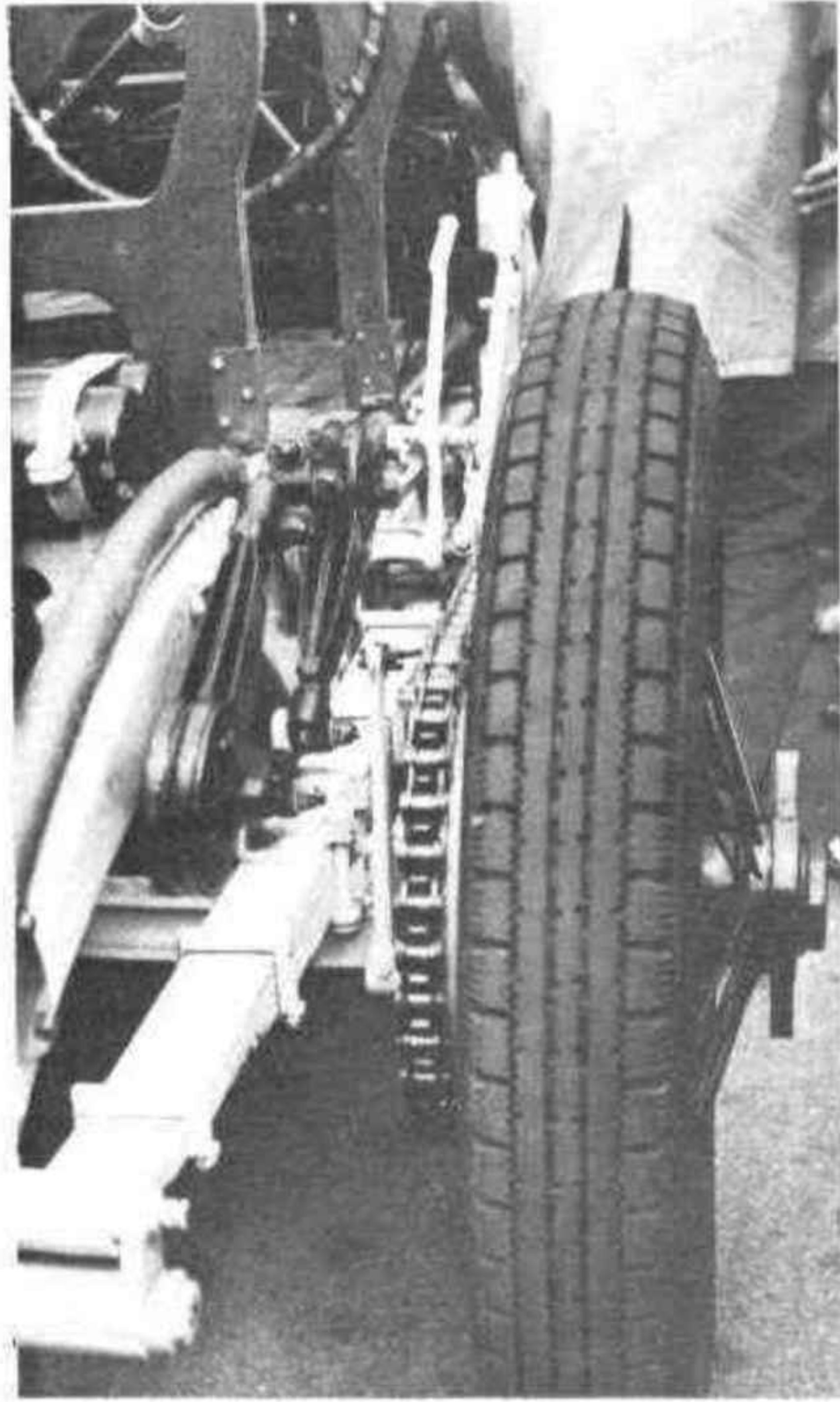
As the picture on the opposite page shows "Babs" sans driving chains, we include this picture of the o/s one, said in 1927, wrongly we think, to have broken and decapitated Thomas. The original sprockets are used.
