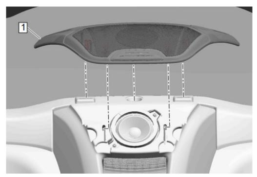
2.) Convertible Models will have an extra body reinforcement bolt/tether that's on the bottom side of the speaker trim, we do not suggest removing this, as you should have enough clearance to push on the backside of the current emblem to remove it from the speaker trim. You may need to use a plastic trim tool to help break loose the edges from the backside of the badge.
