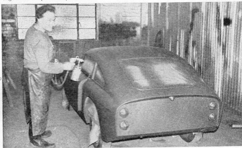
. . . A STREAMLINED 1,100 c.c. Sprite will run in the 12-Hour race as a G.T. prototype by John Colgate and Clive Baker. 95 b.h.p. is claimed from a very reliable engine. The 10 cwt. car has a "plough share" back-end to stop eddies, the front being like last year's machine. . . .
