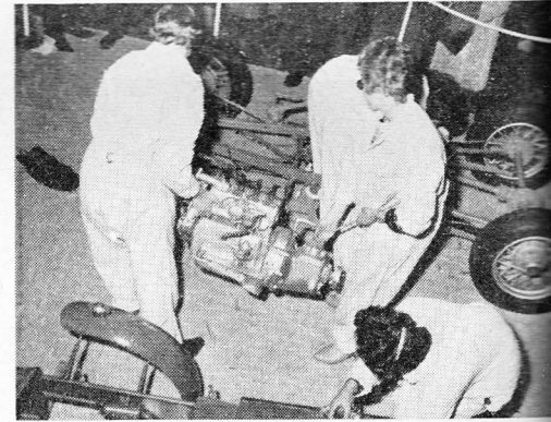
. . . ENGINE and gearbox being fitted. . . .
