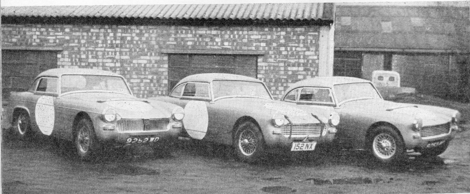
THE MOST works cars ever to go to Sebring from Warwick are, by the time you read this, on their way to America to take part in both the 12- and Three-Hour races on 22nd-23rd March. Left to right (above) are the cars for the latter event: an M.G. Midget for Graham Hill and two Sprites (one is a spare) for an unnamed driver. The cars have aluminium bodywork panels and the 998 c.c. engines develop 88 b.h.p. . . .
