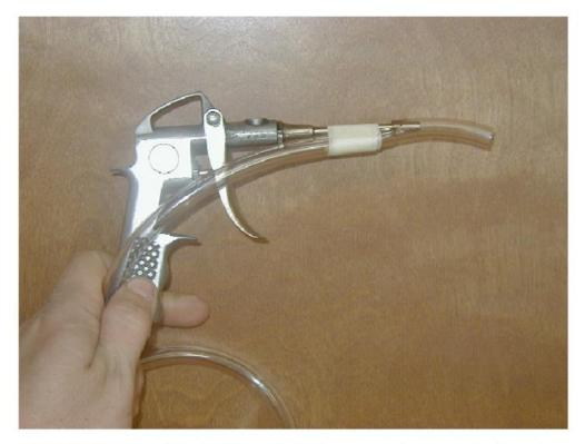
I cut the other end of the vinyl hose at a 45 degree angle to allow better flow of the soda into the hose. Then I tape the piece of dowel, metal rod or wire to the other end of the hose. This will help keep it from curling up in the box of soda and help you keep good flow into the hose. You will need to periodically shake the box to keep the soda flowing nicely.
