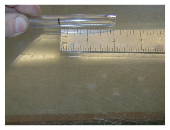
Take your knife or razor blade and make a small cut across the hose ONLY through one side. The cut needs to be just large enough so that the tip of the air wand attachment will stick into the hose. Stick the tip of the air wand into the hose and let it stick in about 1/4" - 1/2".
