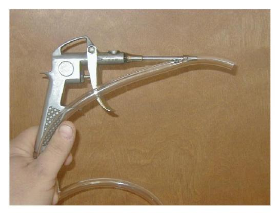
Positioning your wand tip like this will create a venturi effect in the hose causing the soda to be pulled up from the box by low pressure and mixed with the high pressure air from the wand. Use one length of tape to wrap around the end of the air wand and hose. This will keep the hose in the proper position on the wand tip during blasting.
