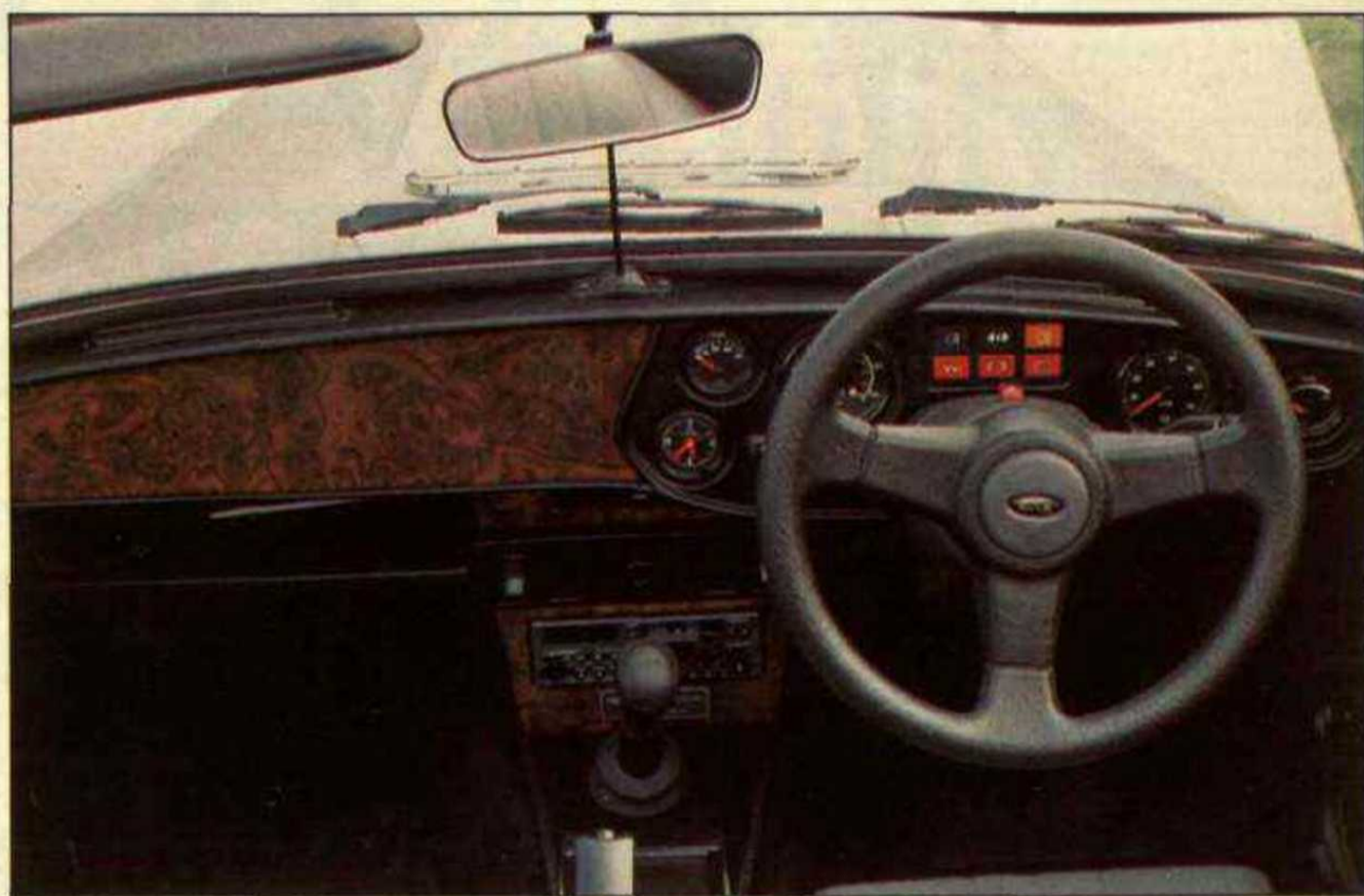
The dash shows five dials, imitation walnut facing and vertical rod from the mirror mounting.
