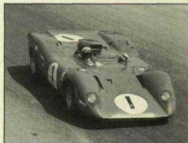
For 1969 Ferrari's long-distance sports-car was the 312P, effectively a Grand Prix car with all-enveloping bodywork.
