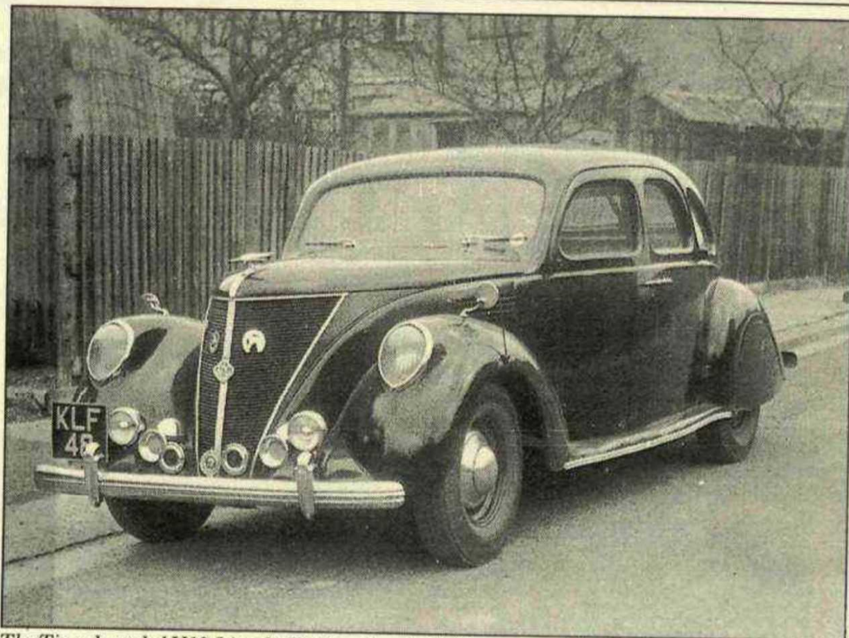
The Tjaarda-styled V12 Lincoln Zephyr, America's first mass-produced unit-construction car.
