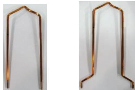
Fig. 5. Hair-pin design before (a) and after (b) twist
