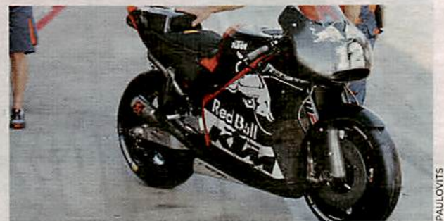
KTM RC16: Gitterrohrrahmen, WP-Federelemente, eigene Formen
