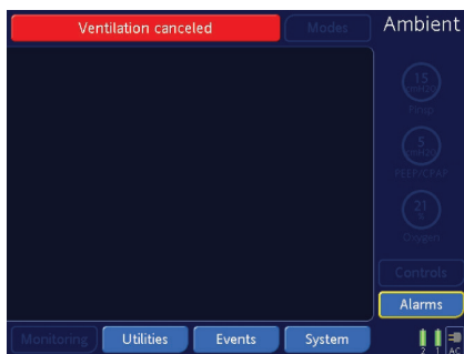
Fig. 12.9 The principle and graphic presentation of the ambient state in the HAMILTON-C2 ventilator.
