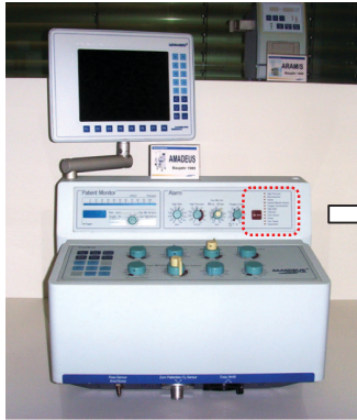
Fig. 12.2 The AMADEUS ventilator has a column of LEDs with predefined alarm messages.
