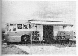
IN THE PADDOCK at Goodwood was the first of the two special vehicles for the Shell-B.P. Racing Service. The vehicles are based on a Daimler fleetline double-deck bus chassis, having special bodywork built by Yeates of Loughborough.
