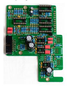
At this point we should clean our board and give the board and us a bigger break. Cleaning boards can be done with alcohol/water/your preferred method. But don't clean the Board after Trimpots, Switches and Pots are installed. Trimpots, Switches, Potentiometers don't like cleaning and that can lead to problems with electrical contact.
