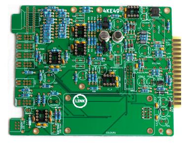
Continue on the LED Meter Board and add all Sockets. Normally we solder first one pin in and trim all of the other Pins as short as possible and continue after that with soldering all other pins on that Board.
