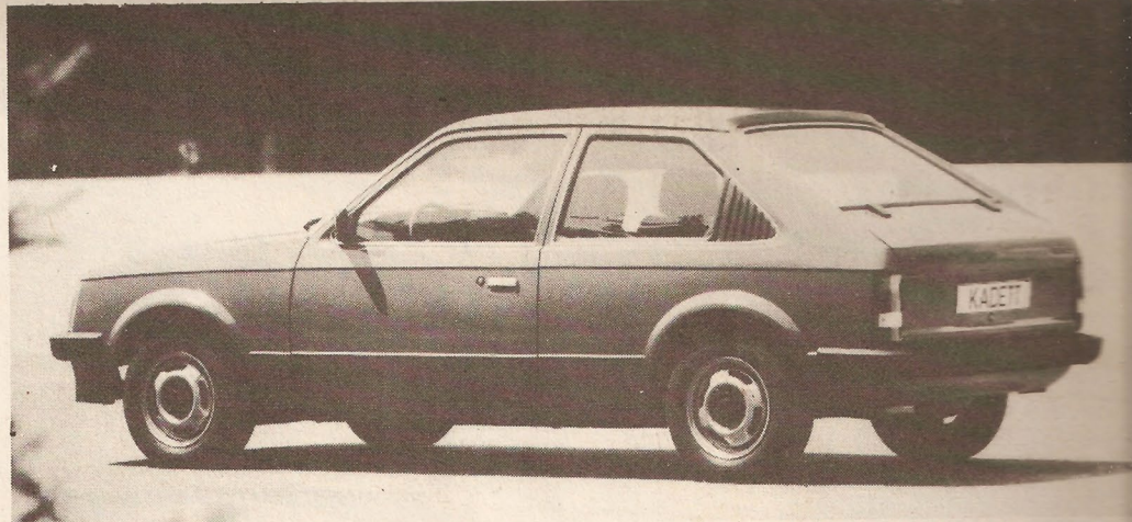
The transverse-engined, front-wheel-drive Kadett is an important addition to the Opel range.
