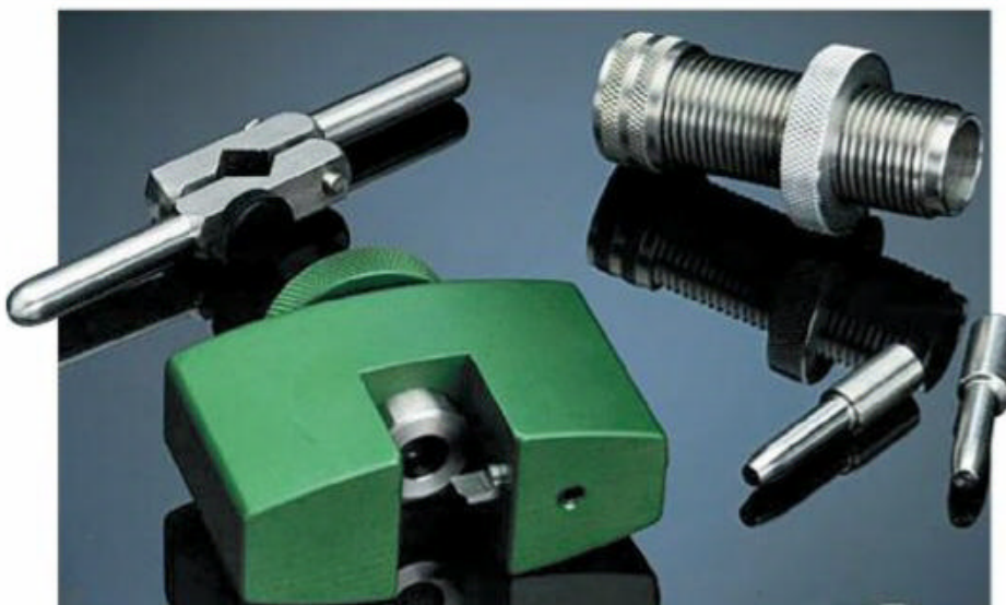
The Sinclair NT-4000 Premium neck-turning tool uses interchangeable mandrels for cases of various calibers. An expander die with a mandrel about 0.001 inch larger than the mandrel of the turning tool is needed.
