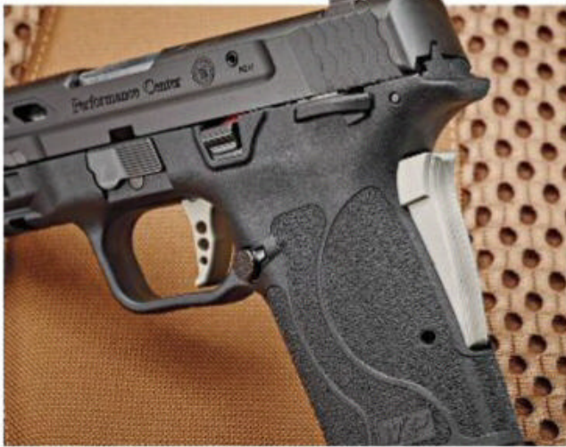
The most distinguishing feature of the Smith & Wesson Performance Center M&P9 Shield EZ is the grip safety lever. It is pinned at the bottom and must be fully squeezed for the trigger mechanism to function.
