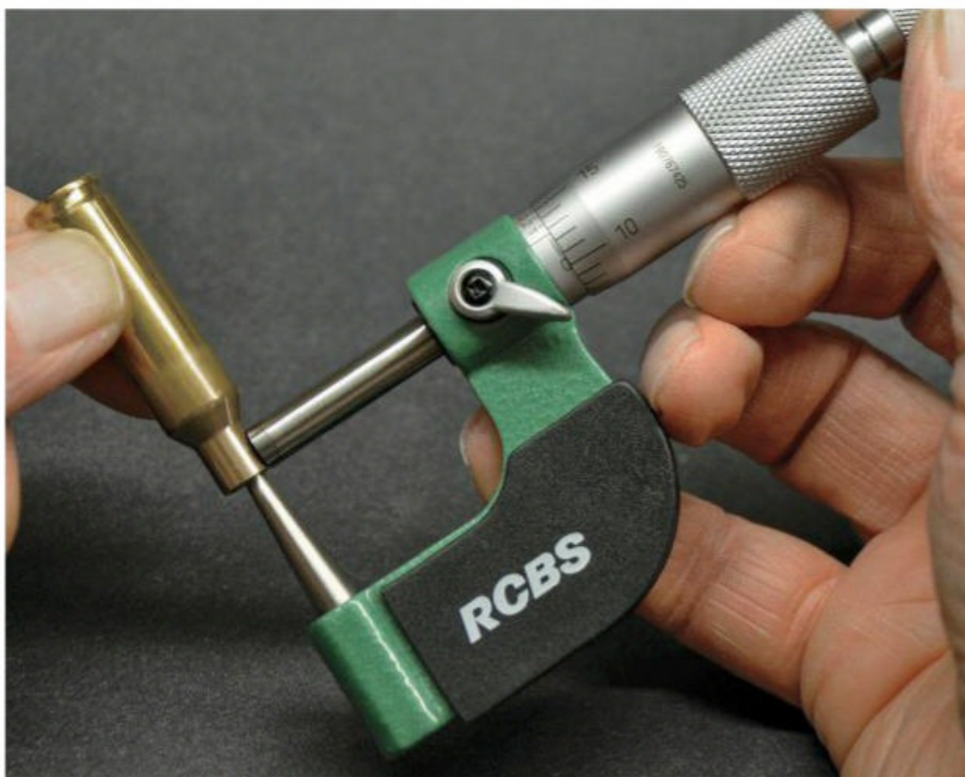
A Vernier ball micrometer capable of measuring to 0.0001 inch is used to check case neck wall thickness and variations of same. It is an essential tool to have when neck-turning cases.
