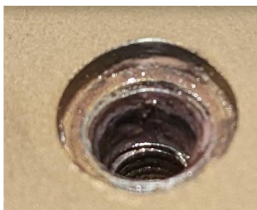
Figure 4: Permanent Chassis Deformation after 40 in-lbf install
