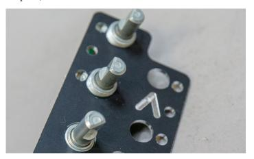
After having all pots screwed to the bracket, we can solder all pins. I cut all the pins before soldering, then they look better, but you can also cut them also after. Then unscrew the board from the bracket.
