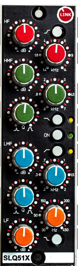
This Switch turns from BELL-MODE into SHELF-MODE of the HF-Band
