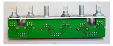
After having one pin of each pot soldered we add the bracket like in the picture shown. The direction of the bracket is shown in the other picture. After having all pots screwed to the bracket, we can solder all pins, after that we need to cut
