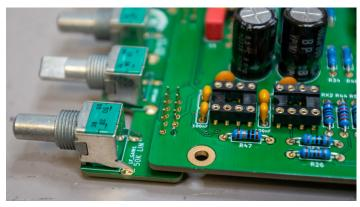
After that we can solder all the other pins and cut the pins also as short as possible. Then you can split our built adapter again in two parts
