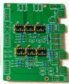
After that Step solder all Wima Capacitors and Board Connections like on the pictures. on the Small Board, the short pins are soldered as close as possible to the board. Its important that you press them in place during Soldering, we need that because of the mechanical assembly later.
