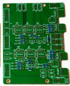
After Placing and Soldering all Resistors, we solder the next bigger parts like IC-Sockets and small Capacitors, like 37x100nF and 16x22pF
