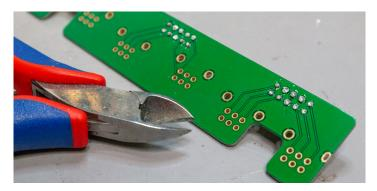
Since we have shortend we install all pots on this board at the same time. get all pots on the PCB and solder just one pin in the middle and press the POT as much as possible on to the PCB. After Soldering one Pin make sure the alignement of the pot is straight. You can check that with printed silkscreen on the PCB.
