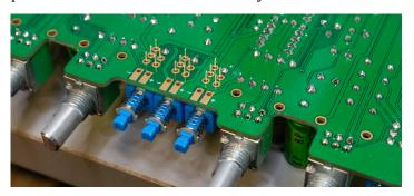
Now we cut the LEDs make sure you have the right leg for + and - ( Long leg is + and short leg is -). I usually cut them not straigt and keep two different long legs that you still know which leg goes to + and -. Make sure the LED is faceing with the forntpanel in one level. First solder one leg to make sure the LED is in place, then solder the other leg. After the whole process, unscrew the Frontpanel and the Bracket, we need that for next step again.
