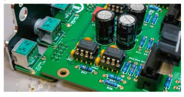
Now we install the upper subboard by adding it angled and connect the ribbon cables at the same process.
