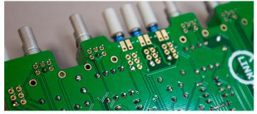
And check again the alignment of the Switches and the pots from upside and try to do it best like the silkscreen is printed. After that install blank bracket on the upper subboard and solder the pots in place.
