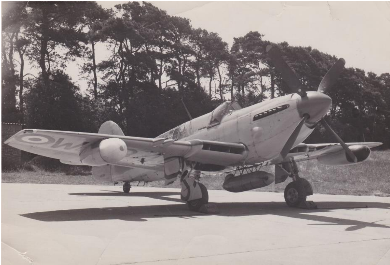
Fairey Firefly FR.5 WB406, D Sqn, Boscombe Down. 5/10/50 arrived for clearance Trials of Liffe "C" type winch. later went to Farnborough for arresting and catapult trials with TT mods. Donald Sellers
