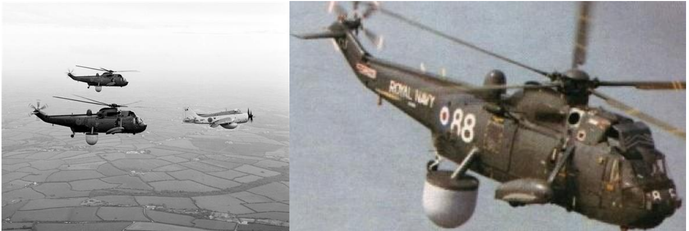
The two Sea King HAS.2' modified for AEW in the summer of 1982, flying alongside the last Fairey Gannet AEW3, returned to airworthiness for propellor noise trials by Dowty Rotor . The second image shows a Sea King HAS2 (AEW) still in its original, pre Falklands conflict colour scheme. Both images FAAM
