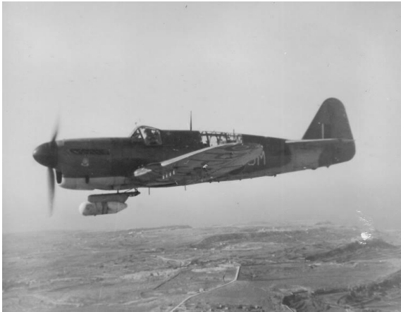
Fairey Firefly FR.I of 816 Sqn . Overflying Malta. The under fuselage Radar, for use in the anti submarine role, identify it as a FR.I. J I Agnew
