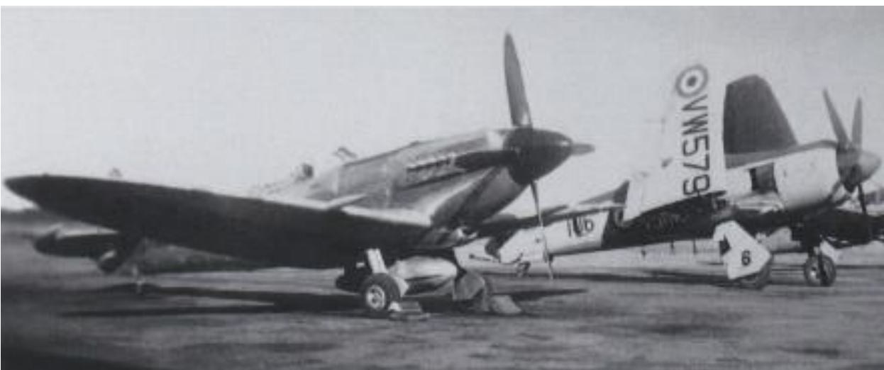
This picture shows Seafire XVII SX161 when in service as The Air Group Commander's aircraft, of the 14 th CAG. It was stripped of camouflage and left in natural metal (not Silver) unlike any others of its kind. Note the flash under the exhaust stubs. The date was 1950 at Hal Far. One of 804 Sqn's newly acquired Sea Furies appears in the Background. Peter Cook
