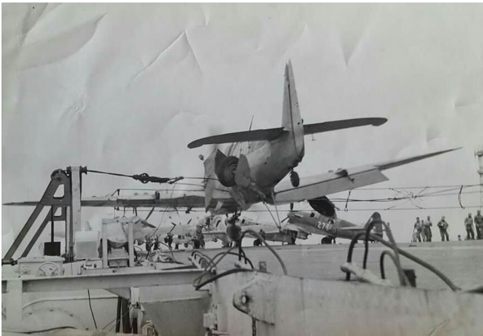
Fairey Firefly FR.5 VT438 812 Sqn HMS Ocean during Deck landing training, Caught an arrestor wire. Port u/c collapsed after hard landing. 13/10/48. Donald sellers
