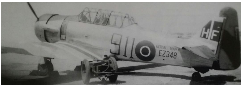
North American Harvard III EZ348 911/HF, Station Flight, Hal Far 1947. The aircraft is natural metal all over, with fabric covered flying control surfaces still in wartime camouflage. mick Burrow
