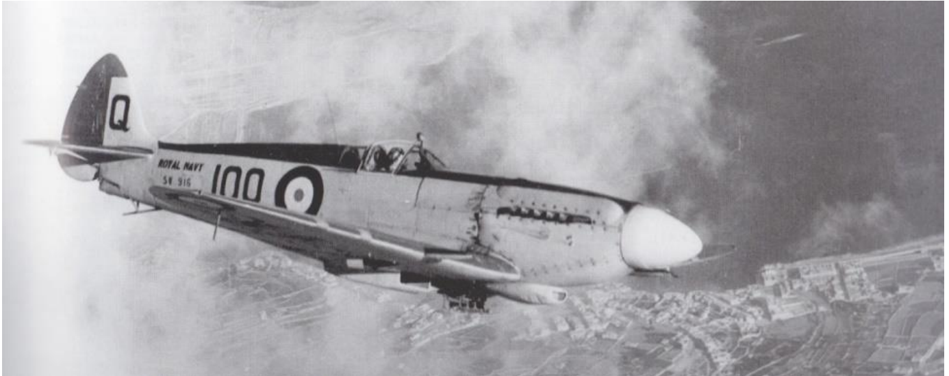
Supermarine Seafire F.XV SW916 100/Q 802 Sqn HMS Vengeance flying over Malta November 1947.note the earlier style canopy.Eddie Fereday
