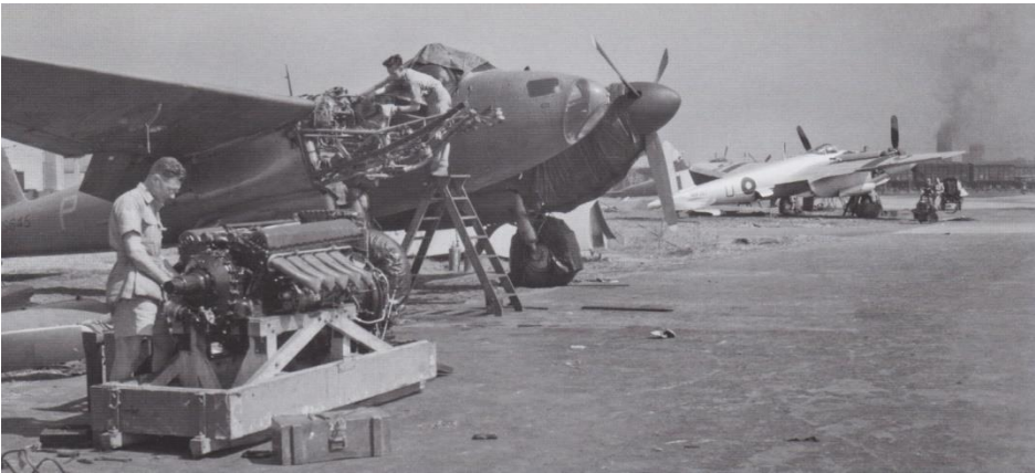
Illustrative picture of, Far East, RAF ground crew , preparing for the physically demanding job of installing a new Rolls Royce Merlin in a Mosquito PR.XVI. Removing one of these was no easy task, weighing ¾ of a ton, and requiring a crane .At least this was possible, outside a hangar, at Hal Far IWM
