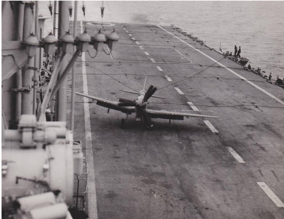
Taken from the "Goofers Deck" of an unknown 804 Sqn Seafire FR.47 landing on HMS Ocean. Note, the LSO screen still not replaced. Donald Sellers
