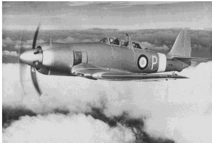
Sea Fury T.Mk 20 prototype VX818 Came to C squadron for trials in April 1951. An ex-Iraqi Sea Fury, this variant first flew on January 15, 1948. Note the strut-mounted periscope viewer for the senior pilot to monitor his student sixty production T.20s were built, and all were land-based and devoid of arrestor hooks. The powerplant was a 2,480 h.p. Bristol Centaurus 18. Web
