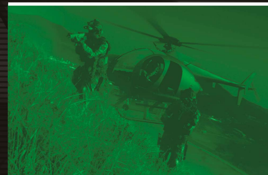
AN MH-9 HUMMINGBIRD INSERTING TROOPS ONTO A HILLSIDE BY HOVERING WITH THE FRONTS OF THE SKIDS TOUCHING THE GROUND
