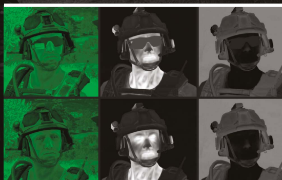
GLASS - IN THE FORM OF COMBAT GLASSES - MASKS THE HEAT SIGNATURES OF THE EYES.
