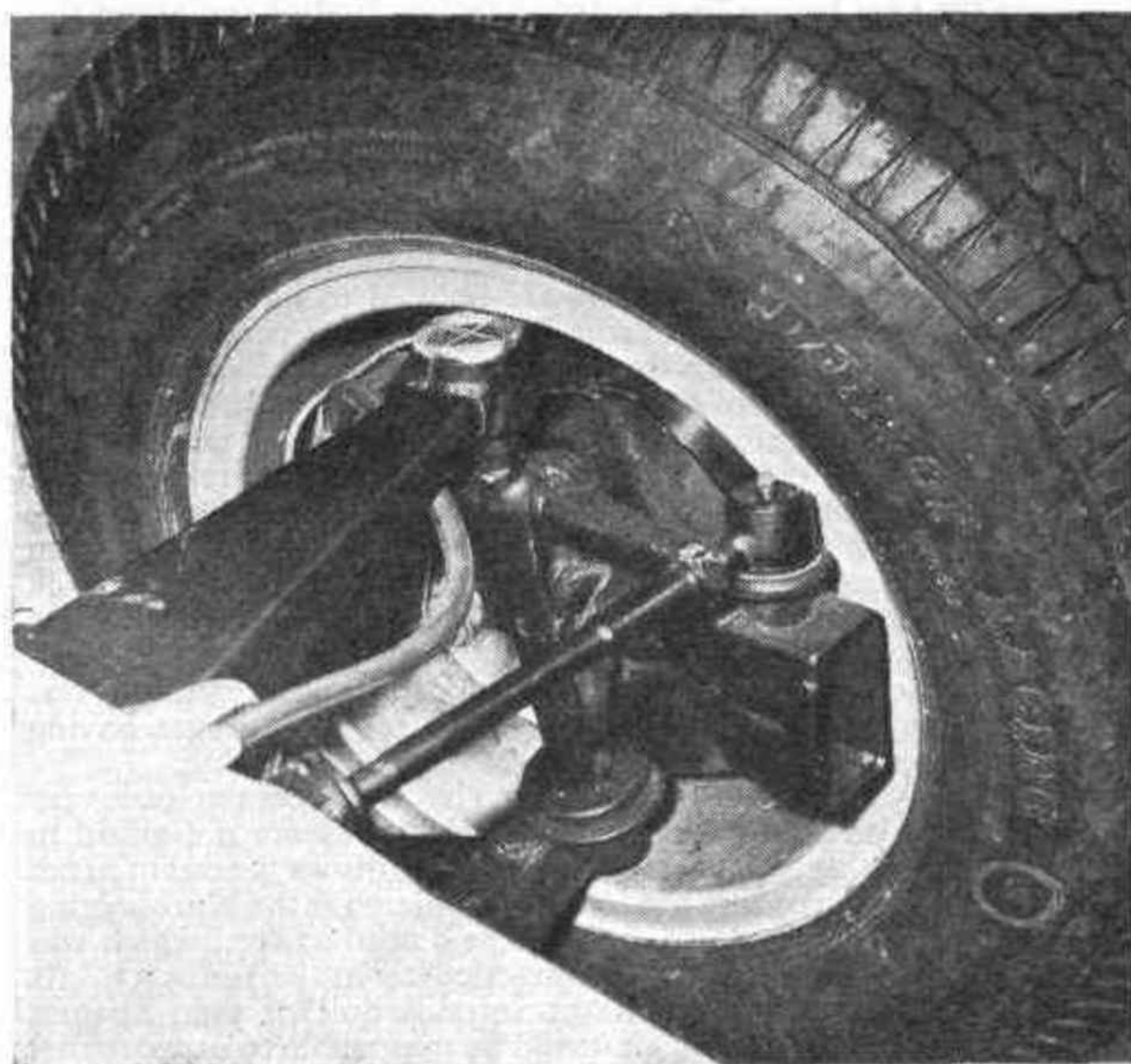
Front suspension of the Honda, which uses a fabricated rocker-arm top wishbone, a forged upright and tubular lower suspension arm. Below the forward-mounted steering arm is an air scoop for the Dunlop disc brake, buried inside the Dunlop alloy wheel.
