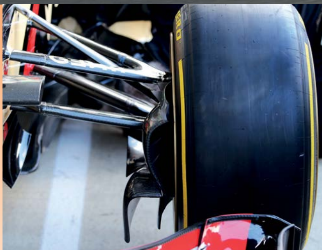
Wheel and tyre sizes have been fixed for a long time in Formula 1, while fans have become used to the aesthetics of low profile rubber elsewhere. Any changes will mean a major rethink in chassis and aero design
