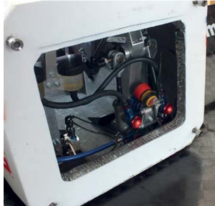
Carbon fibre and aluminium honeycomb sandwich results in a light but rigid chassis structure
