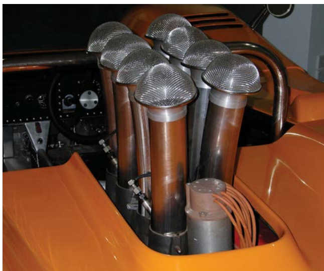
Tall stacks on the mechanical fuel injection. Magneto ignition
