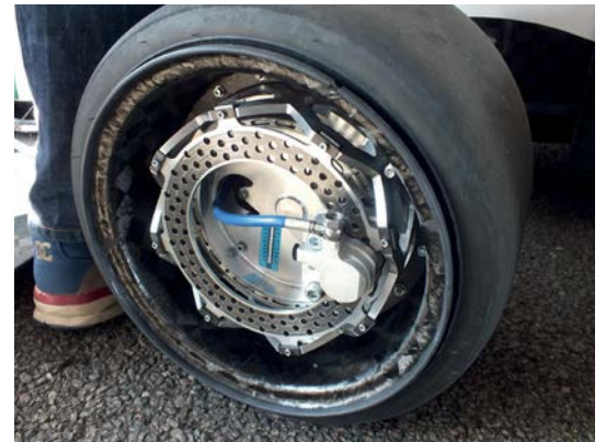
Radical rethink of wheel and hub design looks inside-out but is light and functional. Exposed brake disc gets maximum cooling
