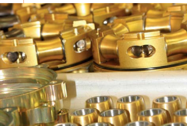
The Citroen WRC roller bearing system, with a specific profile that interacts with the tubes in response to changes in loading
