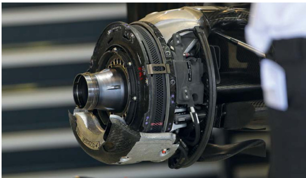
Brakes feature Akebono calipers, but McLaren does not reveal the supplier, or suppliers, of their carbon discs
