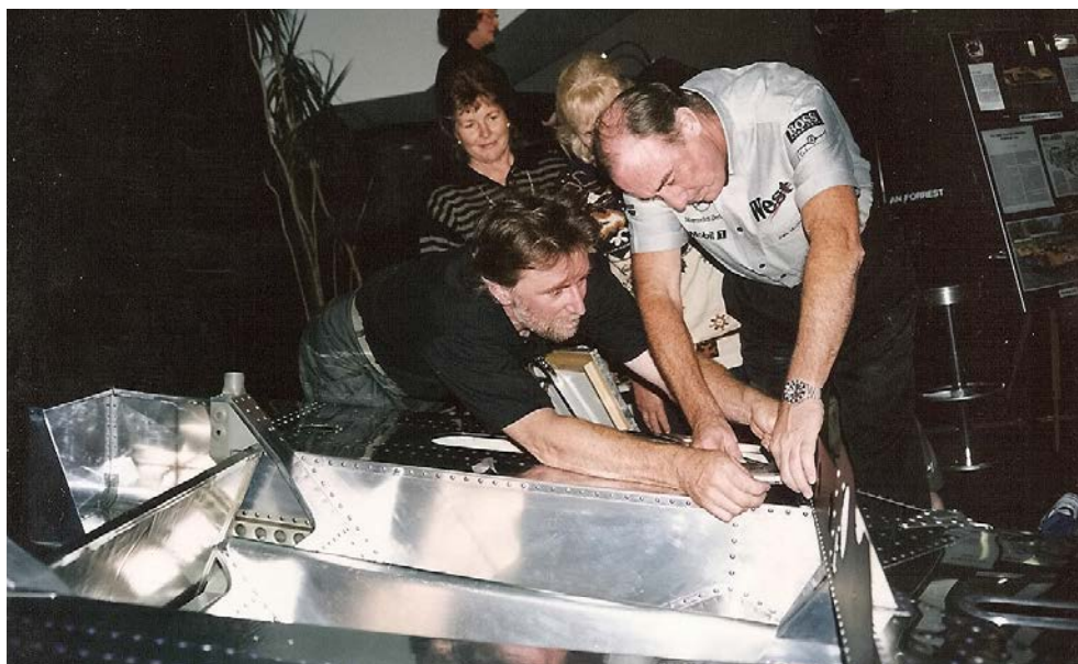
Restoration of the monocoque tub was required due to the deterioration of the inner strengthening bulkheads. Each of the 1000 rivets used in the construction were sourced from the UK to maintain authenticity
