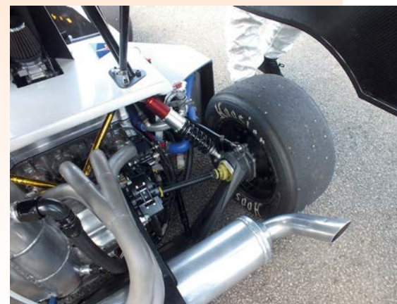
Machined billet block holds Honda CBR internals. De Dion axle with Satchell links removes need for rear subframe
