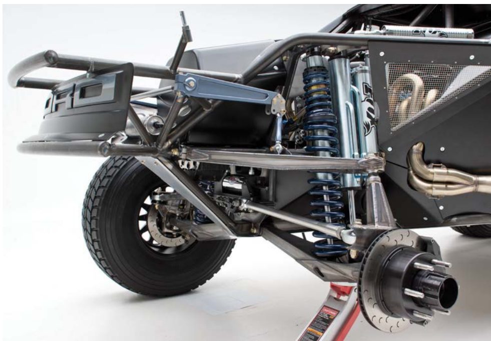
Massive suspension travel and huge tyres dwarf the Alcon 12-inch disc brakes. Surprisingly, two wheel drive is preferred
