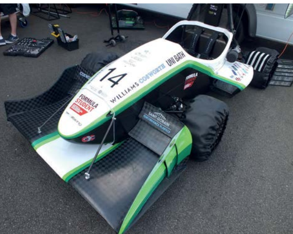
The University of Bath's entry featured an impressive front wing that uses vortex management to improve efficiency. Structure weighs only 3.5kg, but drag would be punitive at higher speeds
