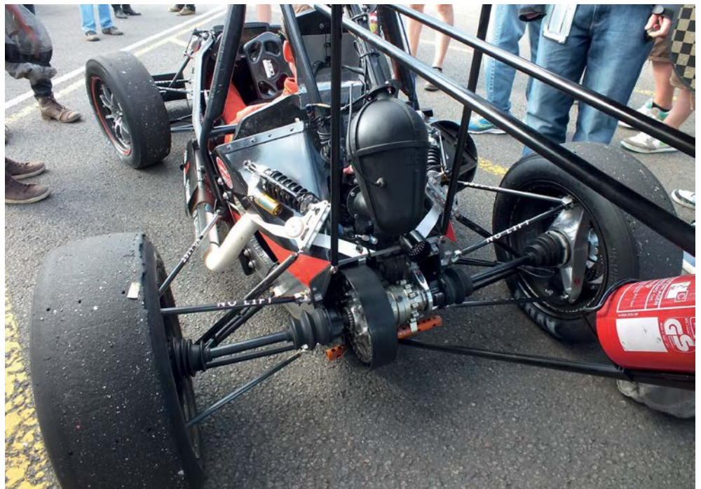
The 570cc KTM single-cylinder bike engine was familiar technology, but the carbon wishbones are all new
