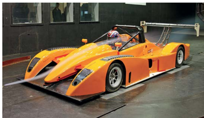
Picture 2: Tiga B, with conventional wing location
