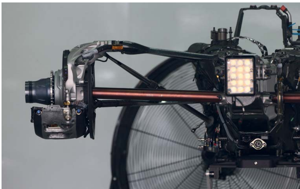
The gearbox and driveline of the McLaren is designed and built in-house and has been one of the most satisfactory parts of the project. This part-assembled view is unobscured by the innovative 'mushroom' wishbones (see box page 12)
