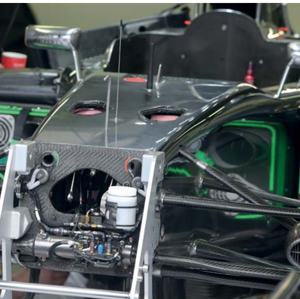
Partly disassembled, a pushrod end is visible through the bulkhead opening. This shot shows the front end without the FRICS hydraulics in place
