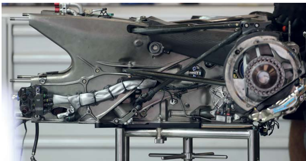
Above: Titanium-cased gearbox is unique to the E22. Full carbon fibre is a future option Right: Experimentation with radiator and charge air cooler placement and ducting is continuing
