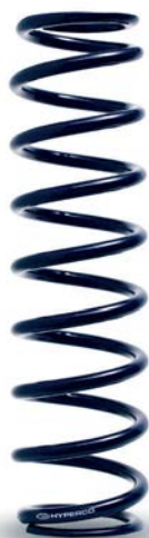
Hyperco's Optimum Body Diameter spring. See how the body diameter increases down the length of the spring, which optimises the applied stress and so the number of coils can be reduced; saving weight
