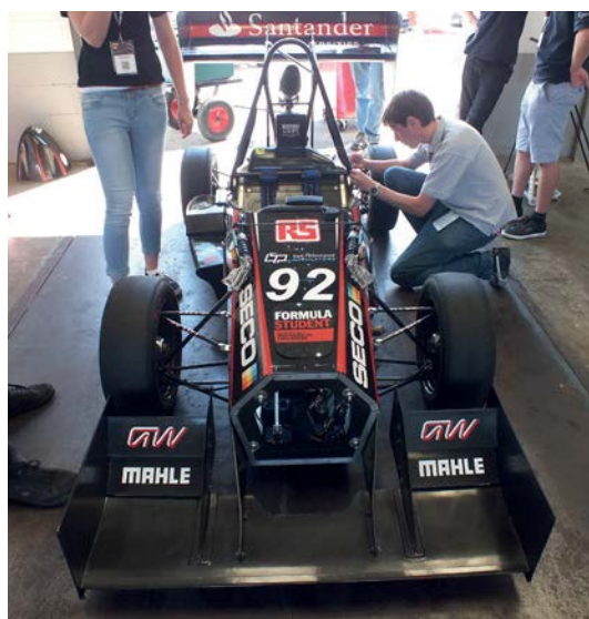
Cost effective folded aluminium monocoque was combined with carbon fibre elements for a significant weight reduction
