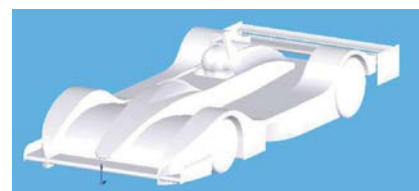
Picture 5: Sports libre model with analogous wing location to Tiga A's standard wing
