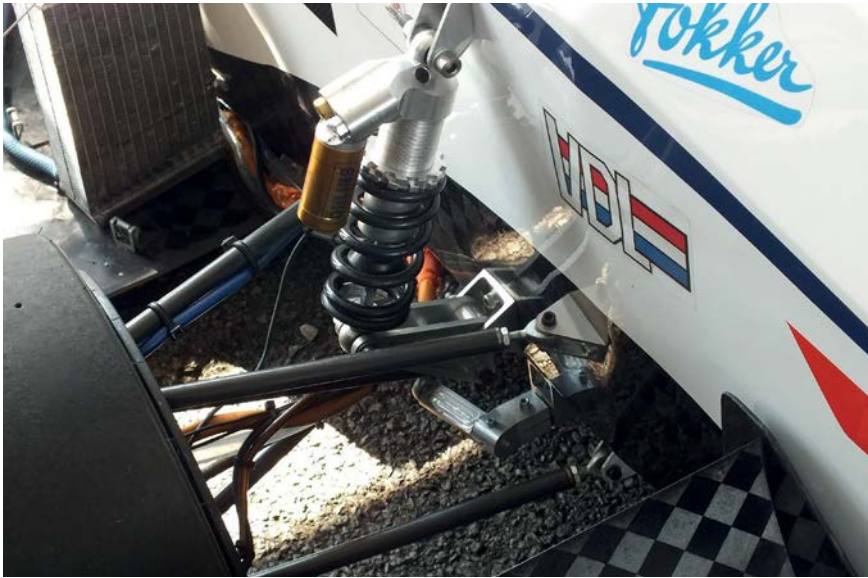
Suspension arm design took 55 iterations before optimisation with the smaller tyre package was achieved
