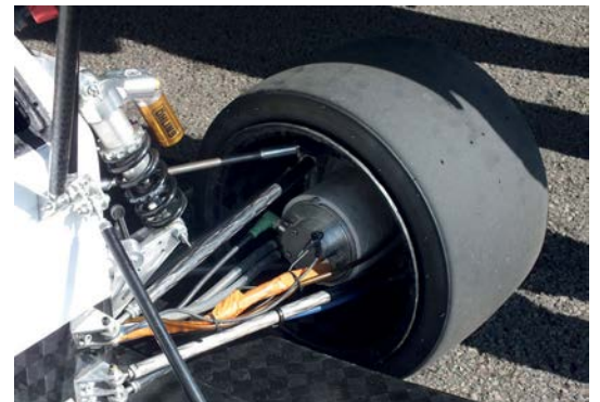
Regenerative braking combines with lightweight lithium polymer batteries to provide efficient energy management
