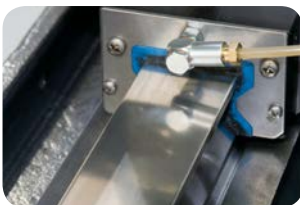
Linear roller guides for high accuracy positioning
