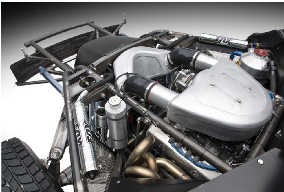
Naturally aspirated V8s from Chevrolet and Ford make about 800bhp, but turbo motors are on the way
