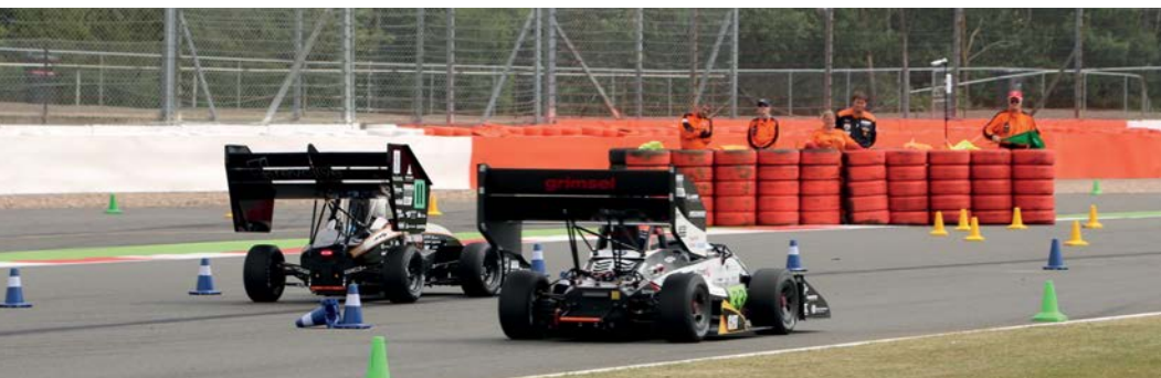
Electric cars, particularly those with four wheel drive, are proving more able on acceleration and can use energy recovery systems, but the acceleration advantage is set to be reduced by proposed rule changes to power outputs
