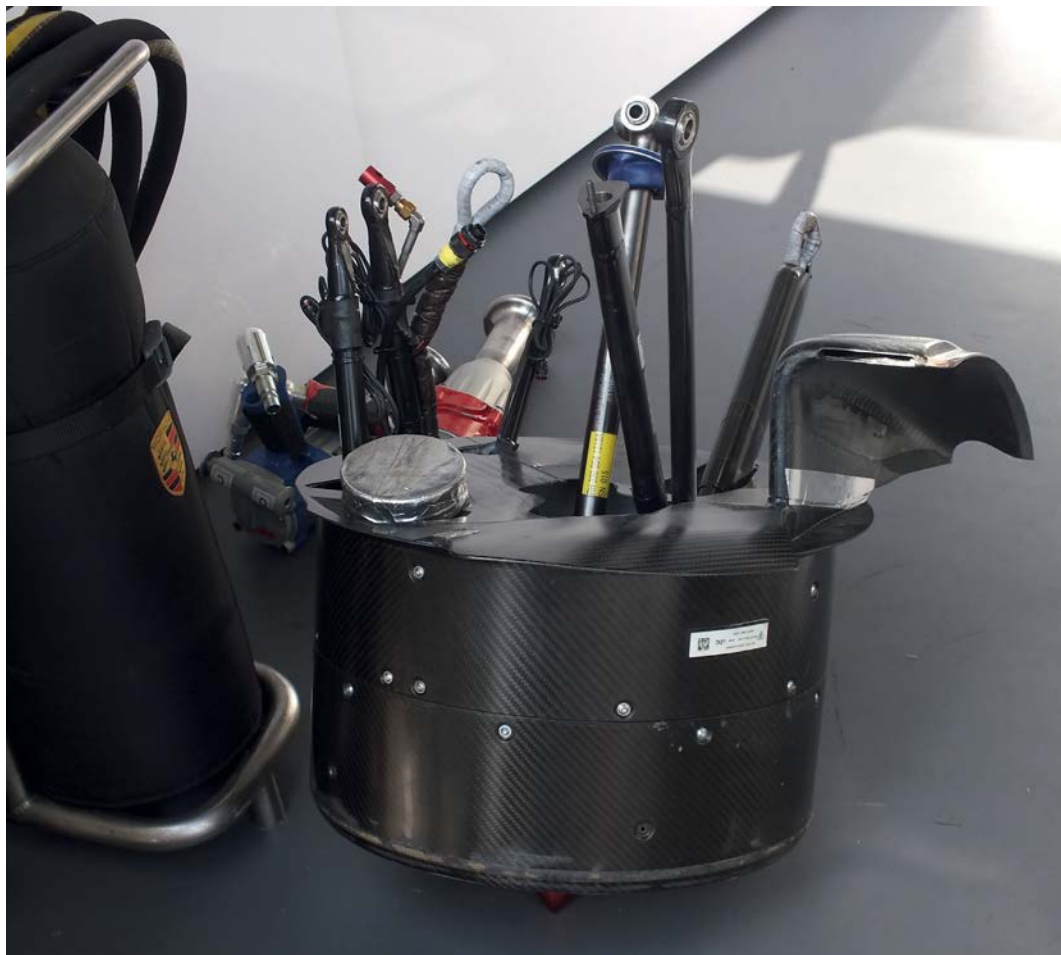
Porsche's suspension assembly for the 919 Hybrid Le Mans car, including the brake shroud and peripherals
