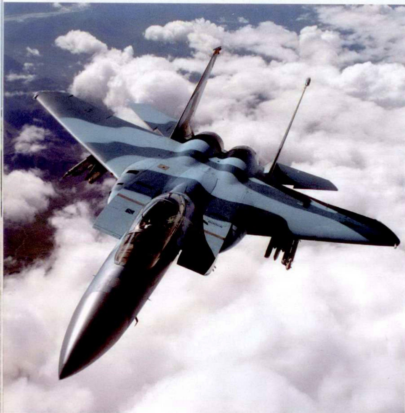
The maximum external load of the aircraft in the air superiority fighter configuration is 6,916 kg and includes three additional fuel tanks and eight guided "air-to-air" missiles. In the case of mounting the AN/ALQ-131 active jamming pod, the aircraft's external load increases to 7,224 kg. The photo shows a two-seat F-15D, whose prototype first flew on June 19, 1979. Photo: USAF
