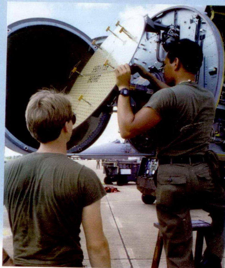
Since 1996, the AN/APG-63(V)1 fire control radar station, which is optimized for air-to-air combat (lacking SAR capability), has been installed on F-15 fighter aircraft. This is an AN/APG-70 station in which many older semiconductor electronic components have been replaced with modern, highly integrated circuits. Photo: Boeing
