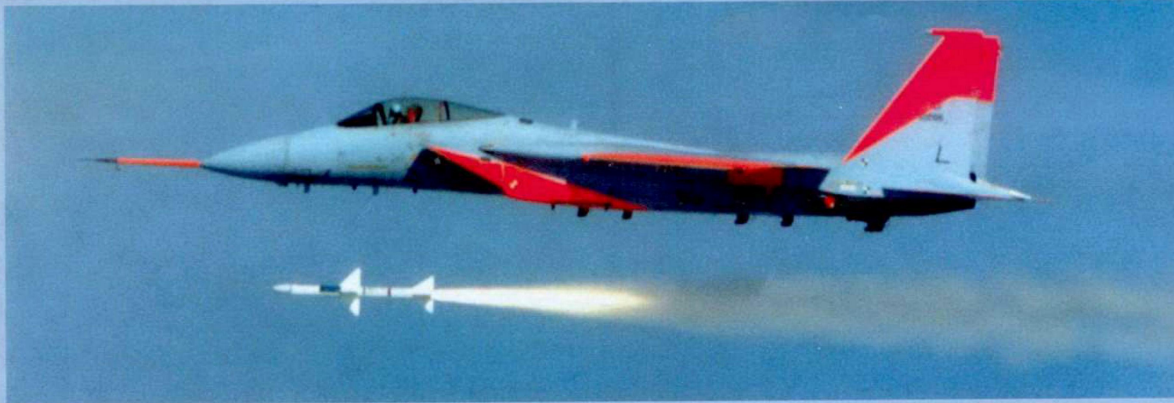
F-15 armament tests: prototype 71-0286 captured during the launch of an AIM-7E Sparrow medium-range air-to-air guided missile (October 1973) and firing the six-barrel M61A Vulcan cannon (August 1974). Photo: Boeing
