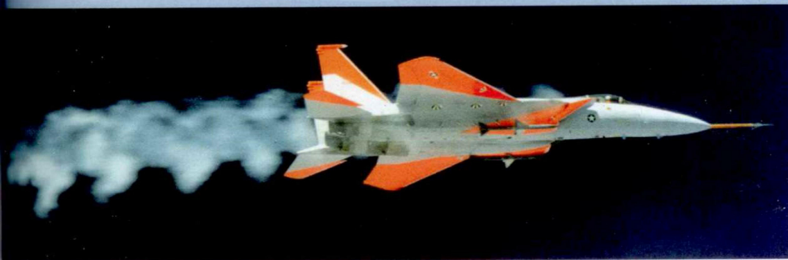
F-15 armament tests: prototype 71-0286 captured during the launch of an AIM-7E Sparrow medium-range air-to-air guided missile (October 1973) and firing the six-barrel M61A Vulcan cannon (August 1974). Photo: Boeing
