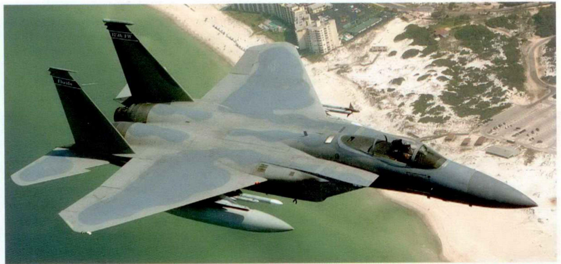
Thanks to its modern and powerful Pratt & Whitney F100-PW-100 engines, the F-15A had a thrust-to-weight ratio of 1.4 at a calculated combat weight of 16,160 kg (this was the average weight at which the aircraft entered aerial combat), and 1.2 at a normal takeoff weight of 19,212 kg (with fuel in internal tanks and armament consisting of four AIM-7E missiles, four AIM-9P missiles, and ammunition for the cannon), both in favor of thrust. This provided it with excellent dynamic and maneuvering characteristics. Photo: USAF
