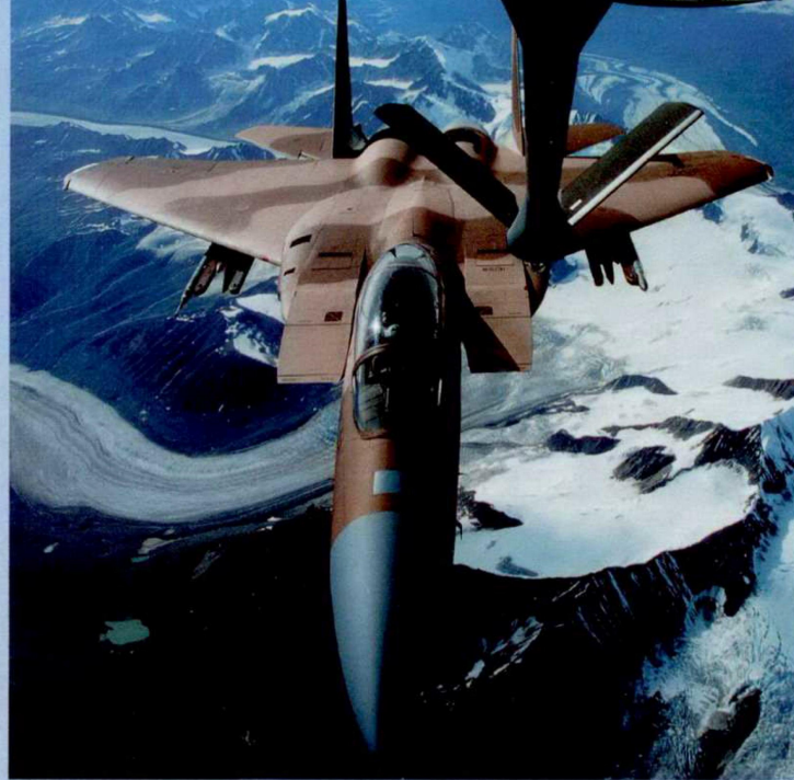
The main area of subsequent modifications was adapting the aircraft to simultaneously engage multiple aerial targets using "air-to-air" guided missiles equipped with active radar homing heads. In the photo - a two-seat F-15D refuels in the air. Photo: USAF
