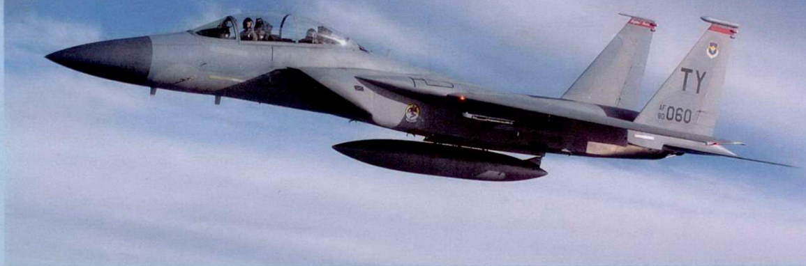
The installation of a second cockpit on the aircraft necessitated the removal of the AN/ALQ-135 active jamming station from its onboard equipment. Placing the station elsewhere was not possible due to electromagnetic incompatibility of the devices. The problem was solved by installing a similar jamming device—the AN/ALQ-131—on the central under-fuselage pylon. Photo: USAF
