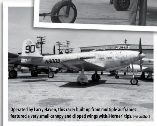
Several P-63 racers were heavily modified, the P-63C, NX62995 the 'Tucker Special' seen here with a remarkably abbreviated wing span of 25 ft 9 in (7.85 metres) cropped by 12 ft 9 in (3.89 metres)! [via author]
