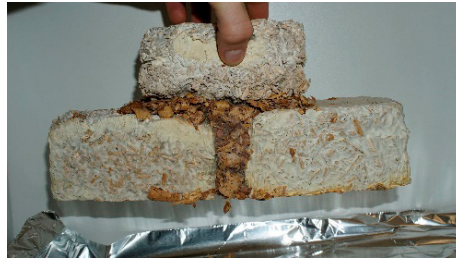
Image 7 - Mycelium paste being used as mortar: In these pictures, the success of the mycelium paste being used as mortar to bind together mushroom blocks is displayed. The mycelium paste has hardened and hooked into the blocks, allowing for the blocks to bind together. This proof of concept suggests further uses of mycelium in masonry construction.
