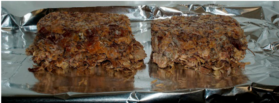
Image 5 - Brown Oyster Mushroom Mycelium and Cedar Shaving blocks: These blocks turned out to be very loose and would not retain their shape.
