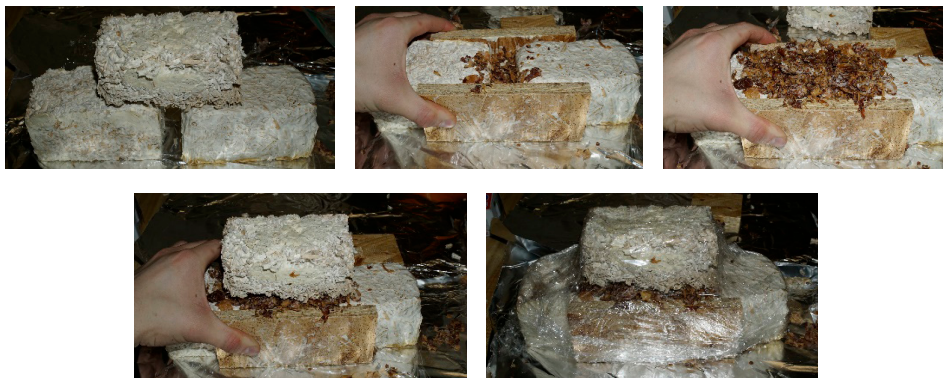
Image 3 - Mycelium block coursing: The mycelium blocks arranged as a half step masonry course with mycelium paste applied as mortar. These blocks measure 3" x 5" x 2.5".
