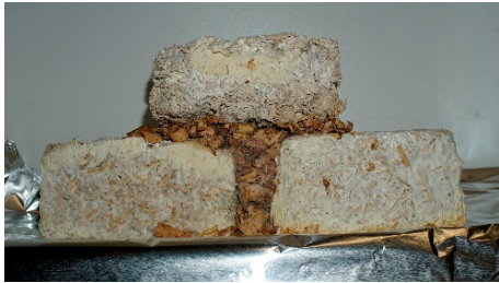
Image 7 - Mycelium paste being used as mortar: In these pictures, the success of the mycelium paste being used as mortar to bind together mushroom blocks is displayed. The mycelium paste has hardened and hooked into the blocks, allowing for the blocks to bind together. This proof of concept suggests further uses of mycelium in masonry construction.
