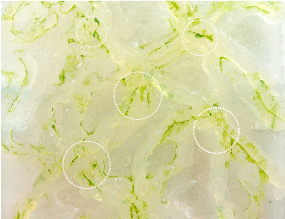
Image 5 - Algae growth test (Irina Shaklova): Algae clusters in hydrogel (Methylcellulose with sodium alginate)
