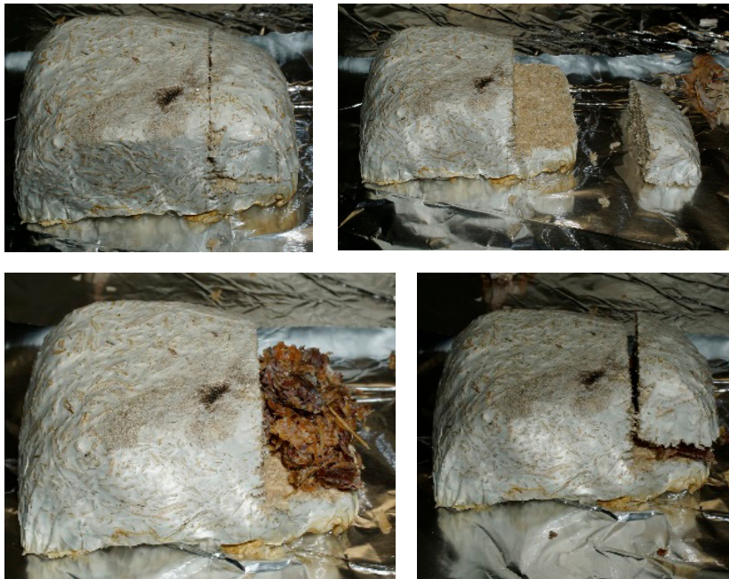
Image 4 - Mycelium block repair: A block that has been artificially damaged and then had mycelium paste applied to the damaged area.
