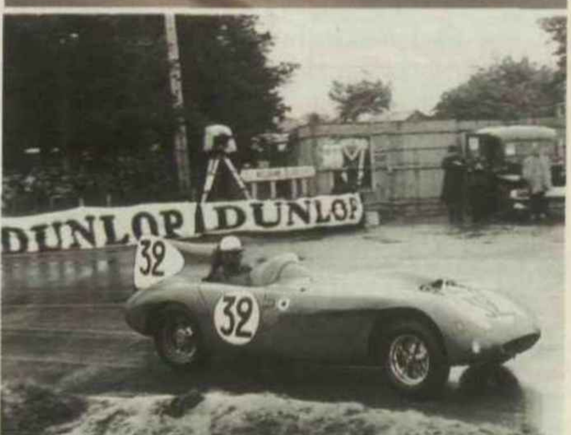
From top: headrest faired into fin; revised coupés took 1954 LM team prize; removal of roof in '55 reduced drag, helped towards repeat team prize
