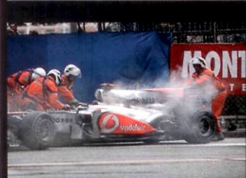
Button retired in Monaco after mechanics left a cover in his sidepod
