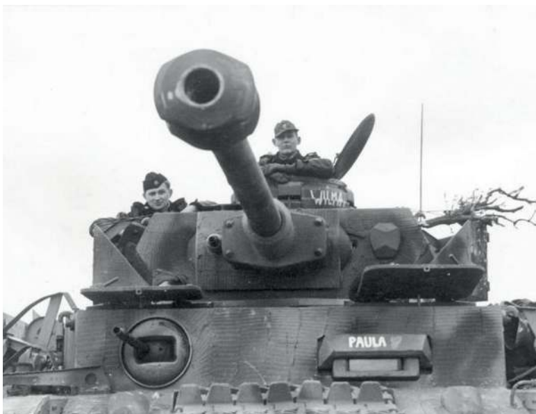
■ A Panzer IV of SS Panzer Regiment 12 in Normandy, summer 1944. The crew have adorned parts of the tank with names of wives or girlfriends. The ridged appearance was Zimmerit paste, applied as a measure against magnetic mines. (BA) Above right: A British Sherman in Normandy, June 1944.
