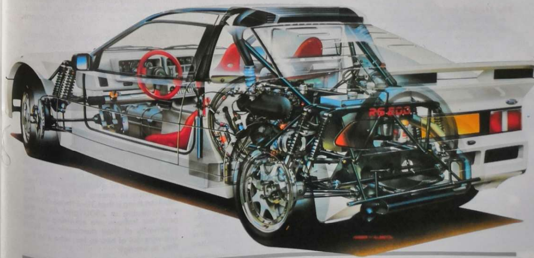
The latest from Ford features a centrally-mounted engine and a front-mounted gearbox. Hence the original transmission layout.
