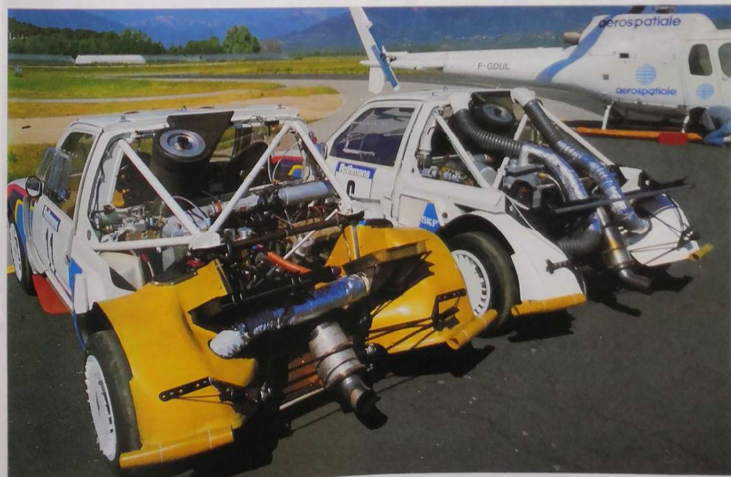
Evolution 1 (right) and Evolution 2 (left) side by side. Note the carbon-fibre covered rear tubular frame.
