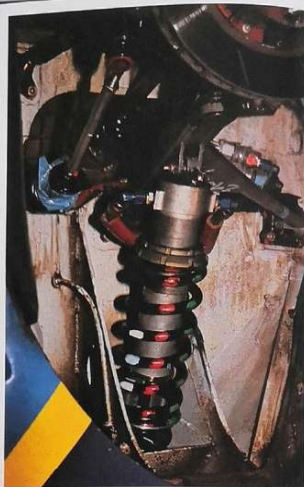
Unique! The front shock-absorbers of the Peugeots were artificially heated in an attempt to conserve their efficiency
