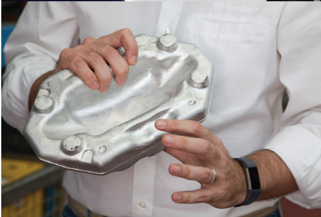
ABOVE & BELOW Race Tech editor William Kimberley was, quite literally, among the first people to see Brembo's B-M6, getting his hands on it shortly after its arrival from the foundry. The calliper is the product of Brembo's innovative 4D-Cast process
