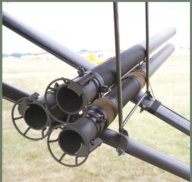
Lt. Rozga was surprised that the blast from launching the rockets had almost no effect on the L-5. He could fire them one at a time or in salvo mode. (Photo courtesy of James P. Busha)
