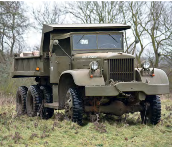
ABOVE: Some time during 1943 production swapped from the hard cab to the military style open cab allowing greater visibility
