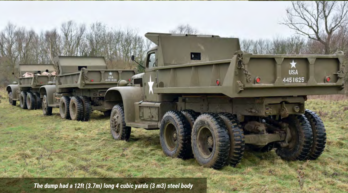
Three variants in reverse order; open cab with winch, open cab, closed cab
