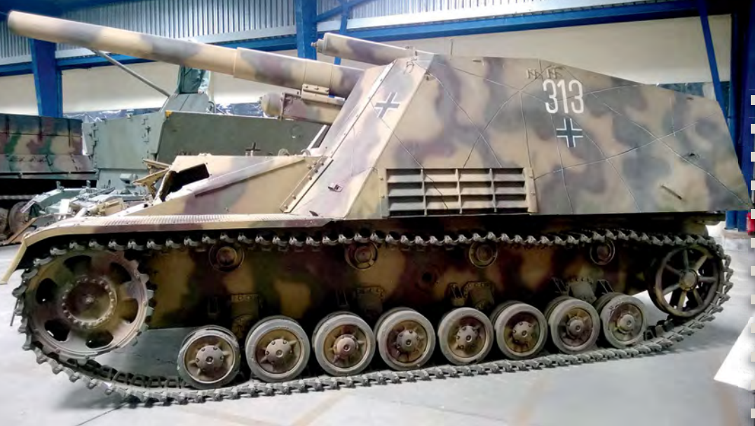
The Geschützwagen III/IV tank hull was slightly longer than the standard Panzer IV tank hull allowing for more room for the driver and passenger
