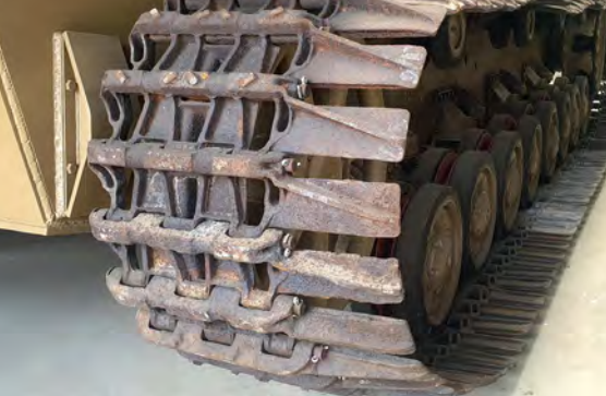
To the left of the track, there is a curved piece of metal attached to the hull side. This is a track pin bump. Track pins were kept in place by a split pin on the outside edge of the track. AUSTRALIAN ARMOUR AND ARTILLERY MUSEUM
