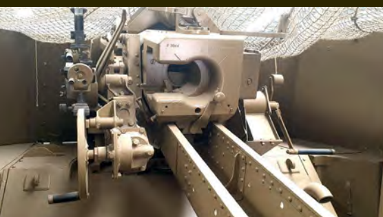
The Hummel was fitted with a 15 cm s.FH 18/1 L/30 heavy field howitzer and could carry only 18 two-part rounds. AUSTRALIAN ARMOUR AND ARTILLERY MUSEUM
