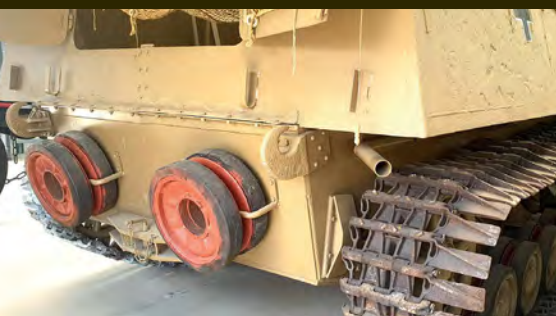
On early Hummels, there was an exhaust silencer box attached to the rear of the vehicle under the hatch doors. Gun crews got burnt. AUSTRALIAN ARMOUR AND ARTILLERY MUSEUM
