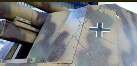
The Hummel at the Museum of Armour (Musée des Blindés), in Saumur, France has black lines painted over the upper superstructure. This is to simulate wire the crew would have strung around the vehicle to hold in place tree and bush branches to help camouflage the vehicle
