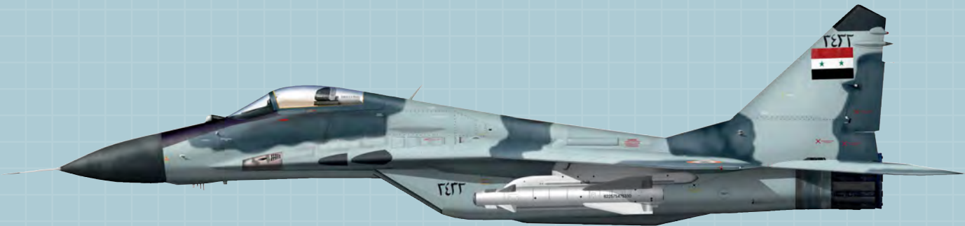
Above: In 2013-14, MiG-29s upgraded to SM standard flew a number of combat missions with Kh-29 (AS-14 'Kedge') guided missiles to deliver precision strikes on insurgent headquarters and bridges. This small fleet is now compatible with Izdeliye 190 (R-77) medium-range air-to-air missiles.
