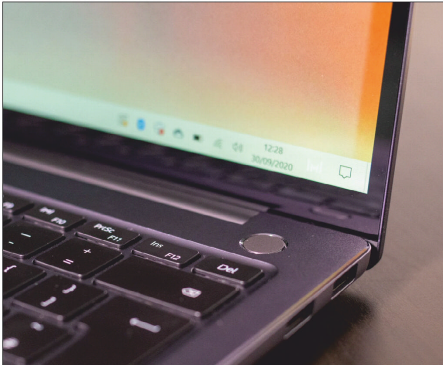
A fingerprint sensor is embedded in the power button.
