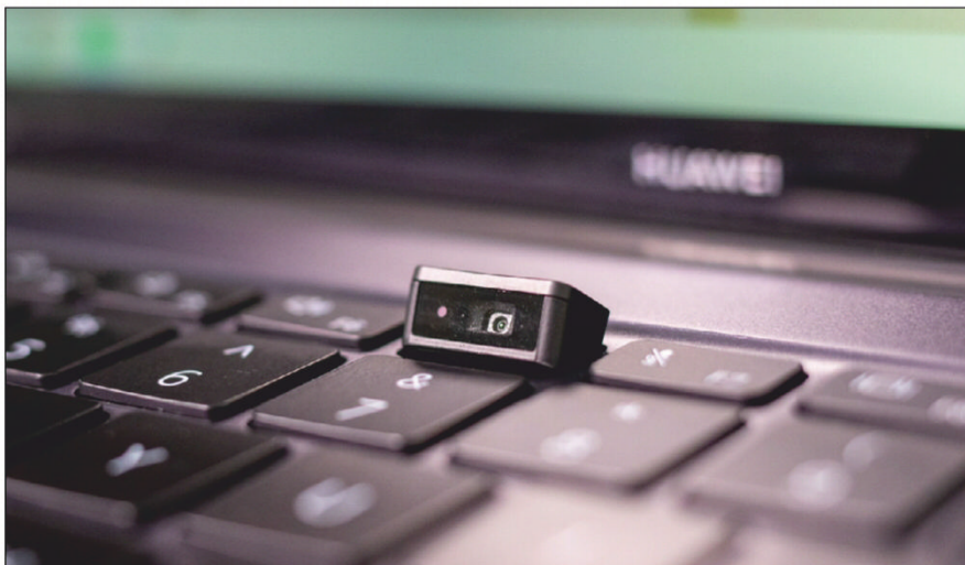
The keyboard includes Huawei trademark: a hidden webcam.
