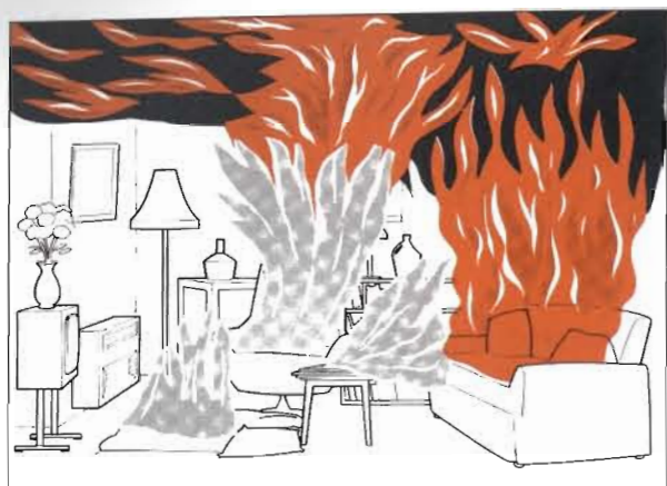
Figure 3.3 Rapid Heating of All Combustible Materials
