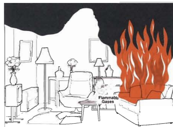
Figure 3.1 The Build-up of the Smoke Layer
