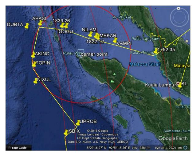
It so happens that the distance between the 19:41 ring and ISBIX via UPROB is the same as the one posited above for the intersection of the path reversing from the 20:41 ring at a ground speed of 470 kts. Based on these parameters, the BFO calculated for 19:41 is 111 (as measured).
