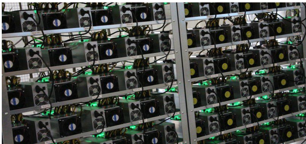
Figure 6. Cooling system & arrangement of hardware. Two large diameter fans decrease pressure inside the container, resulting in directional inflow of cool air through ventilation ducts. Archive racks on rails are used to host the hardware.
