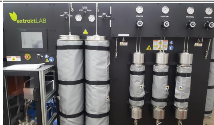
Figure 14: CO2 extraction equipment
