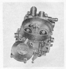
TWIN-CHOKE Solex carburetter was one of the most interesting on view, being effectively two carburetters together.
