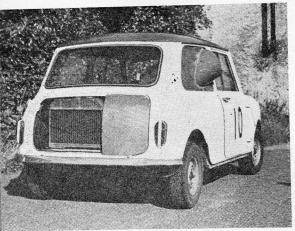
REAR VIEW of the extraordinary device shows the D.K.W. radiator in the boot and air scoop on the offside.
