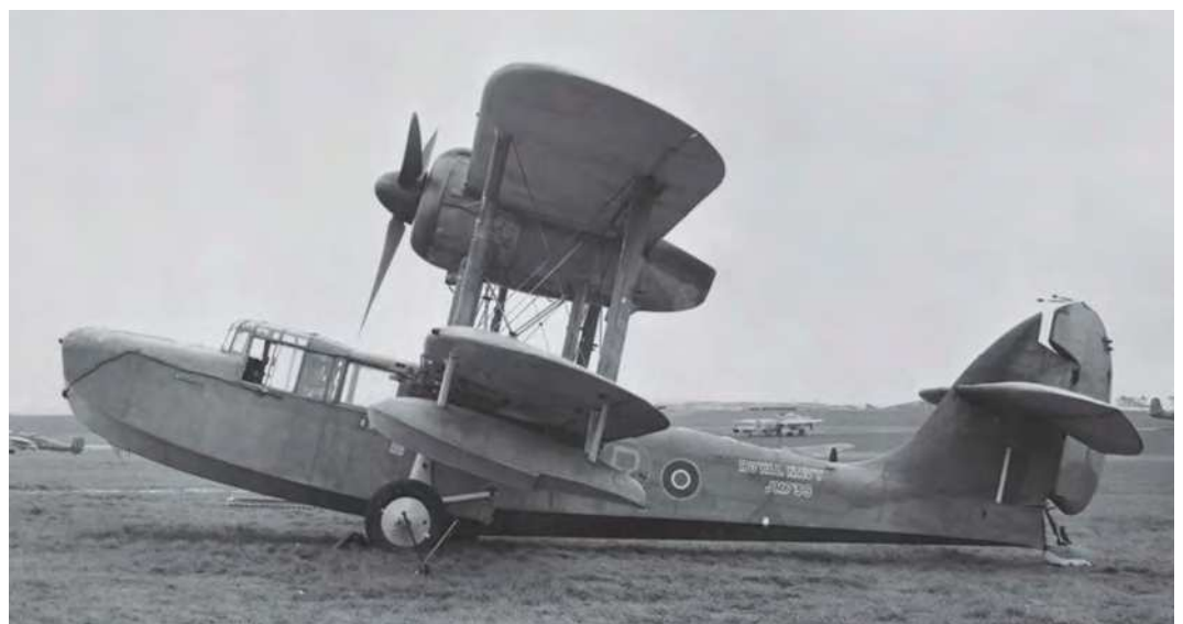
TOP: A good view of the 'scissor' propeller arrangement on Sea Otter K8854, which proved necessary to fit within the height requirement and to part company properly from the water. KEY COLLECTION ABOVE: Sea Otter ABRI JM739 marked for testing with the prototype 'P'. CROWN COPYRIGHT
