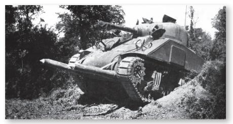
The attack on the Martinville Ridge on July 15–16 by the 29th Division was supported by specially modified tanks of the 747th Tank Battalion, fitted with two timber prongs on the bow to create cavities in the base of hedgerows. After impaling the timber prongs into the hedgerow, the tank withdrew and accompanying engineers filled the cavities with prepared explosive charges to blow gaps into the hedgerows.
