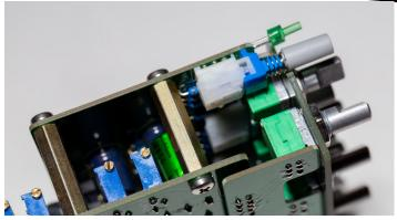
Now it's time to add the Frontpanel to complete the Equalizer. Use the spacers and the M3 Nuts to finish it. The Caps for the Knobs are sorted as following:
