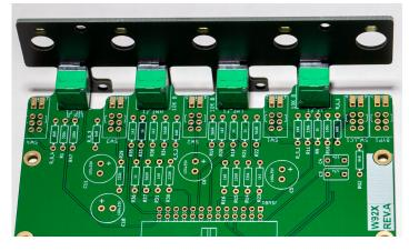
After having one pin of each pot soldered we add the bracket like shown in the picture above. The direction of the bracket is shown in the picture below. After having all pots screwed to the bracket, we can solder all pins, then we need to cut the pins.
