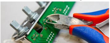
The next step is focusing on the pots and switches of the upper subboard, we can solder all pots and switches. Make sure to press them flush and firm to the poard and fix them with one solder point.
