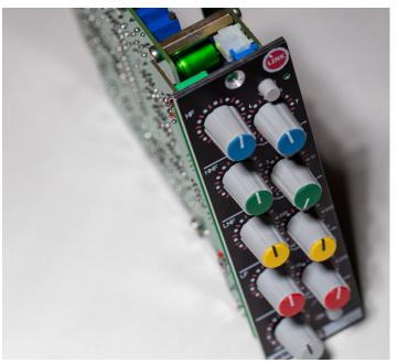
After finishing try to run an Audio Signal thru the Unit and try all switch modes, if everything works fine. If you have a bump when switching the Low or Highcut Filter, don't worry these filters need to be calibrated to have the right level. Try also if all Gains and Frequency Pots are working. You can do that either in the measure software or with Audio Signals. In the next step we will calibrate this wonderful Equalizer.
