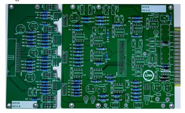
After Placing and Soldering all Resistors, we solder the next bigger parts like IC-Sockets and small Capacitors, like 100nF Caps
