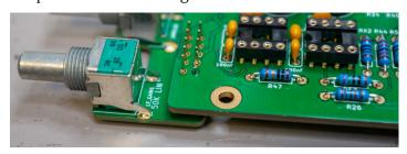
After that we can solder all the other pins and cut the pins also as short as possible. Then you can split our built adapter screws in two parts again.
