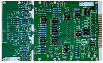
After that Step solder all Wima Capacitors and Board Connectors like on the pictures. On the Small Board, the short pins are soldered as close as possible to the board. Its important that you press them flush in place during soldering. We need them to sit flush and straight for the mechanical assembly later.
