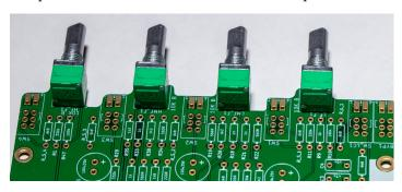
Check the alignment of the switches and pots from the upside again and try to bring them in line like the silkscreen is printed. After that install the blank bracket on the upper subboard and solder the pots in place.
