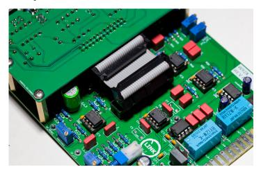
Now we install the upper subboard by holding it angled and connect the ribbon cables at the same time.
