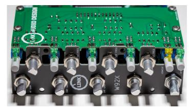
Then check all ICs for the right orientation again. Next put all the ribbon cables on the mainboard.
