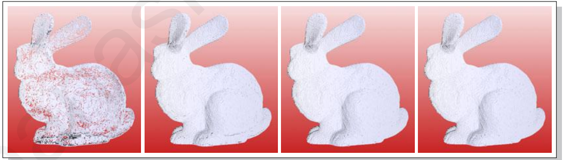
Figure 66: Comparison of the voxelization using the pixel shader clipping method at 256^3 volume resolution with 3, 6, 9 and 12 geometry shader vertices output. The number of voxels produced are 52382, 87690 and 89696 (complete voxelization) for 3, 6, 9 and above geometry shader output vertices, respectively.
