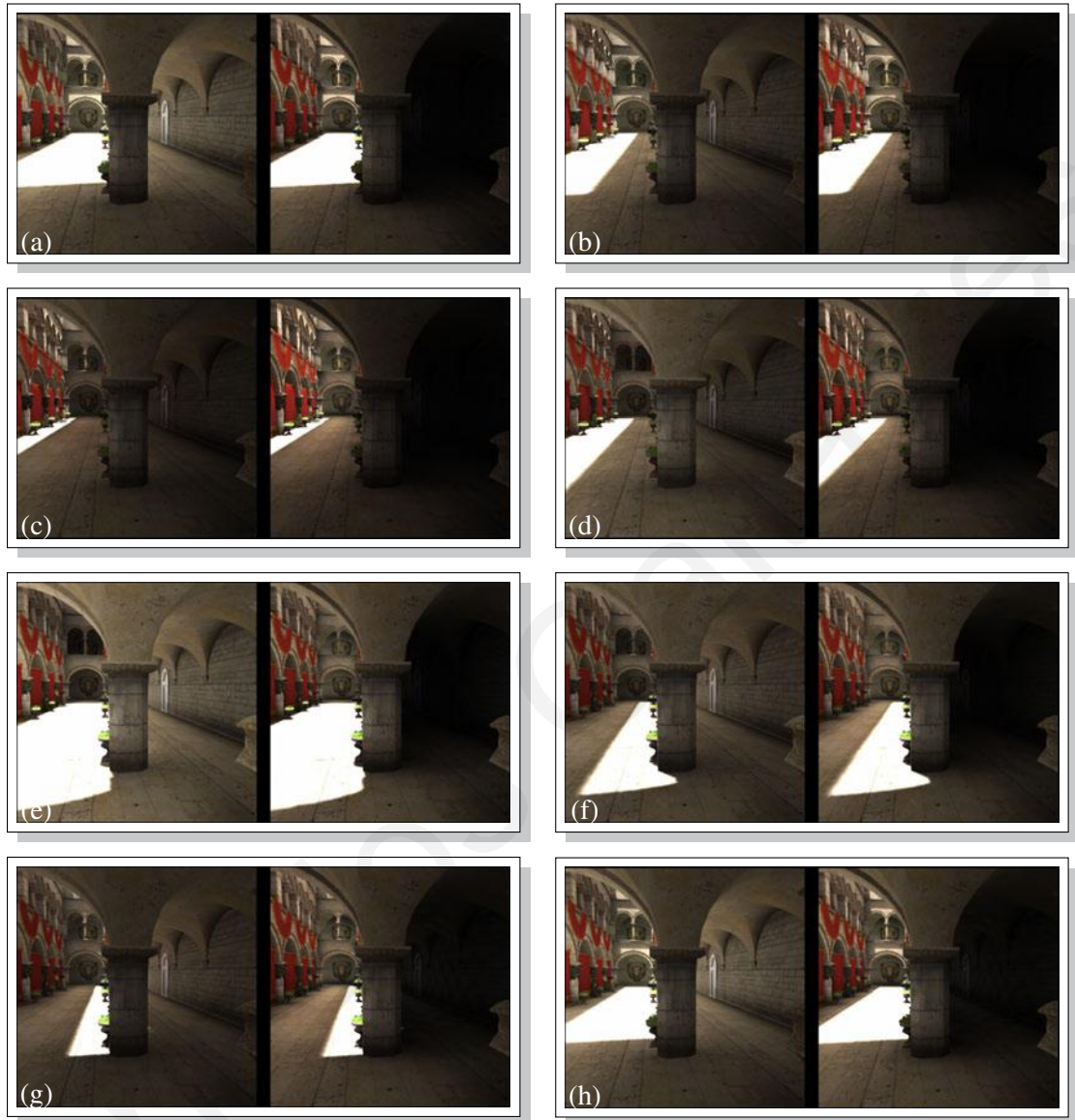
Figure 79: Scene with dynamic lighting. Sequence of a side-by-side comparison of a single-frame image-based voxelization (left images) vs. incremental image-based voxelization (right-images). The curtains that are hidden behind the colonnade do not obstruct the light in the case of the single-frame voxelization.
