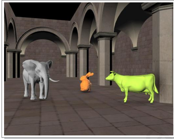
Figure 41: A scene of the Sponza Atrium with a bunny (38889 tris), a cow (92864 tris) and an elephant (157160 tris) rendered in three passes (one per object) with the visibility fields algorithm using 4226x64x64 maps and rendering in 2.5 frames per second.
