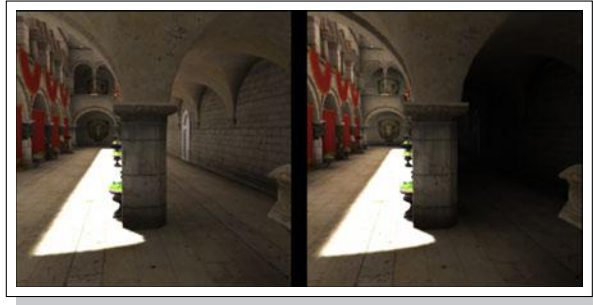
Figure 5: Side-by-side comparison of a single-frame image-based voxelization (left inset) vs. incremental image-based voxelization (right inset). The curtains that are hidden behind the colonnade do not obstruct the light in the case of the single-frame voxelization.
