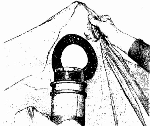
Placing Envelope over Shaft [29]
