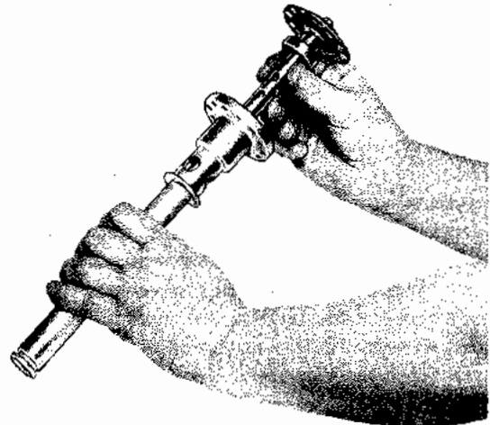
[152] Installing Valve in Housing
