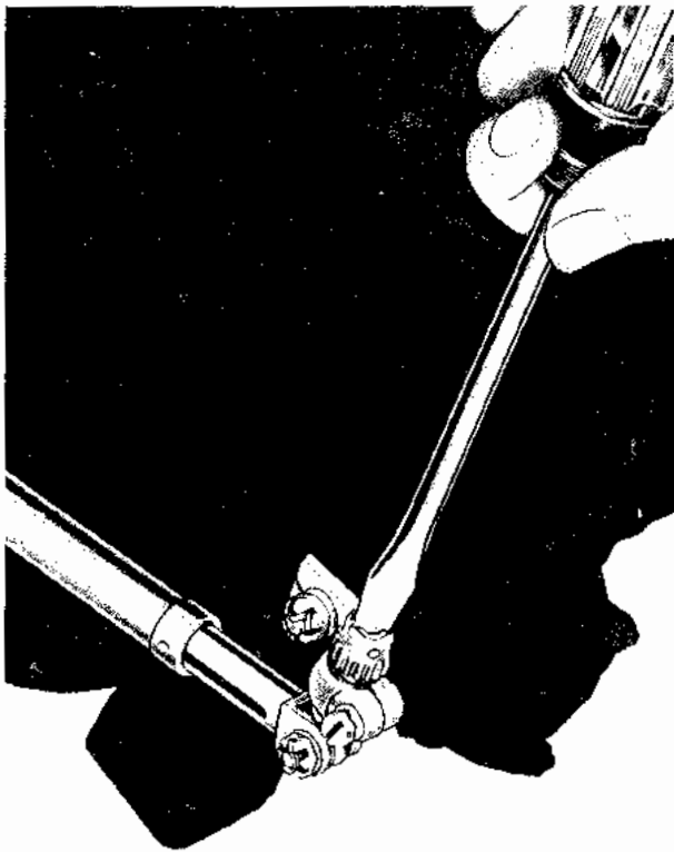
[43] Adjusting Idle Mixture
