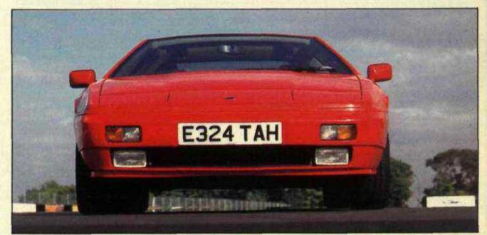
Turbo's inset spot-lamps help reduce drag by cutting the volume of air through the radiator.
