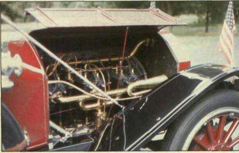
Three separate ignition systems operate a total of 18 spark plugs.
