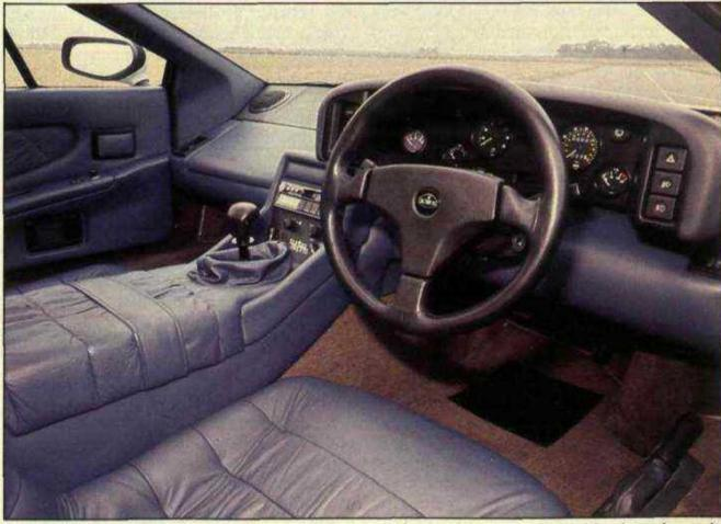
New binnacle is more rigid, and trim quality is tighter, but awful handbrake position is unchanged.
