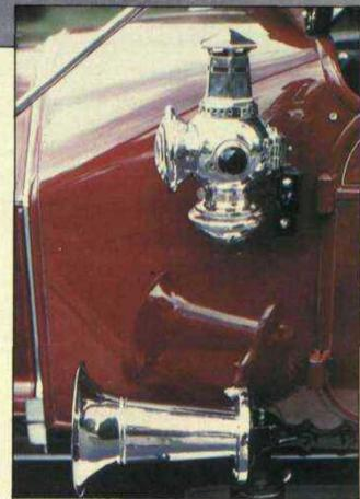
Scuttle-mounted lamps converted to electricity.
