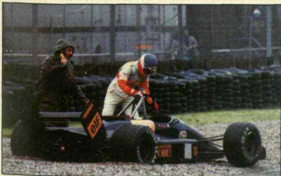
The AGS's rear-wing collapsed nine laps after start-line damage . . .
