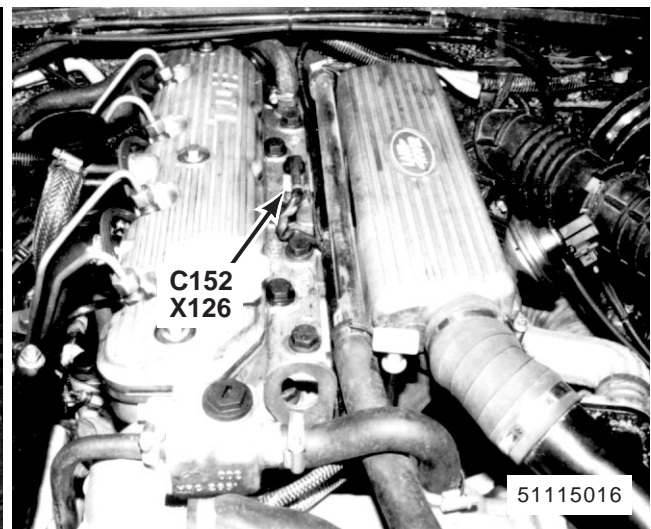
20. top centre front of engine (300Tdi without EDC) X126 Engine Coolant Temperature Sensor C152 (2-N)
