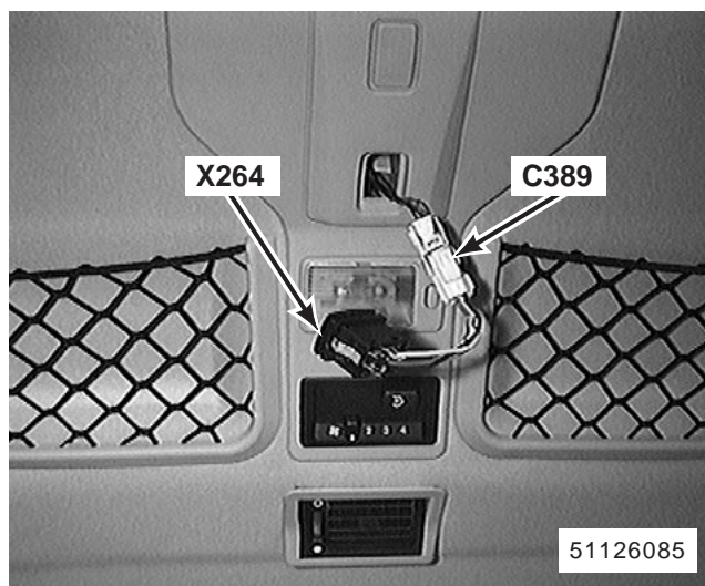
198. centre of roof X264 Passenger's Rear Sunroof Switch C389 (3-W)
