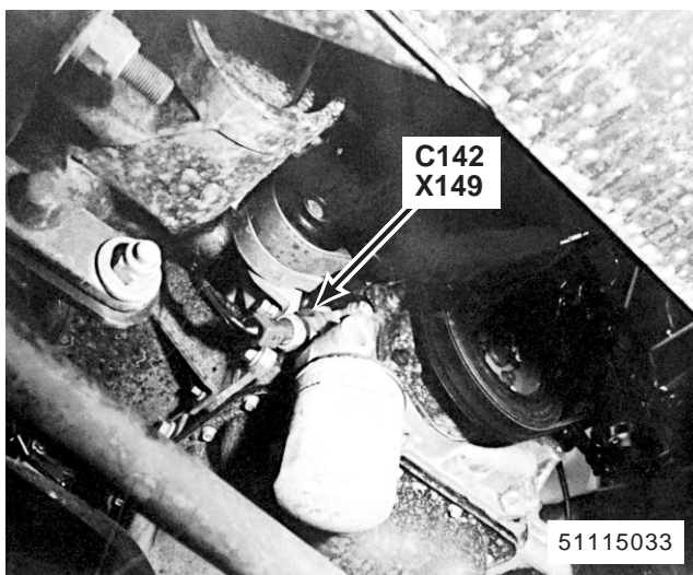
40. lower RH side of engine (MFI-T16) X149 Oil Pressure Switch C142 (2-N)
