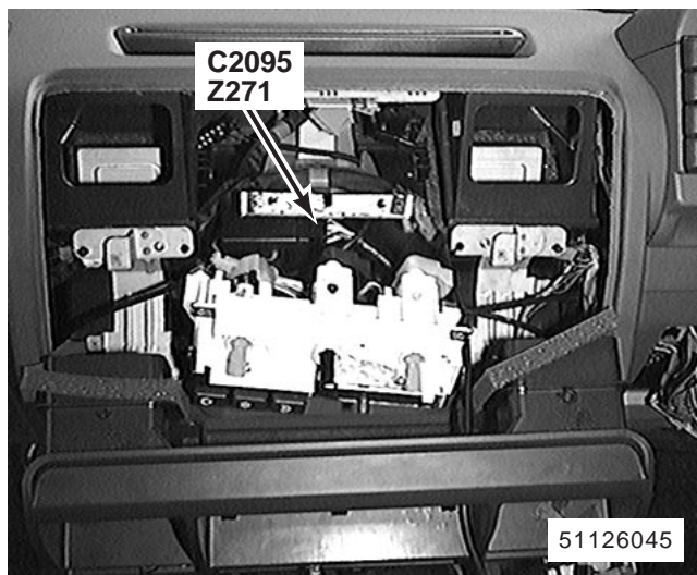
119. behind centre of fascia Z271 Engine Immobilisation Control Unit (Spider) C2095 (9-B)
