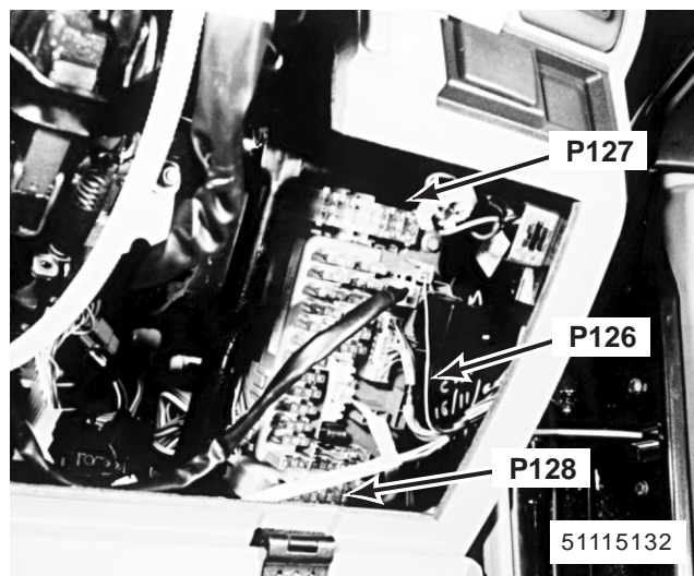
160. behind RH side of fascia right of steering column P126 Fascia Fuse Box P127 Satellite Fuse Box 1 P128 Satellite Fuse Box 2
