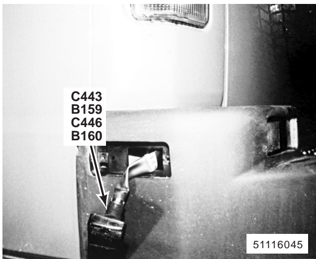
223. behind LH side of rear bumper (RH similar) B159 Left Rear Side Marker Lamp B160 Right Rear Side Marker Lamp C443 (2-B) (Left) C446 (2-B) (Right)
