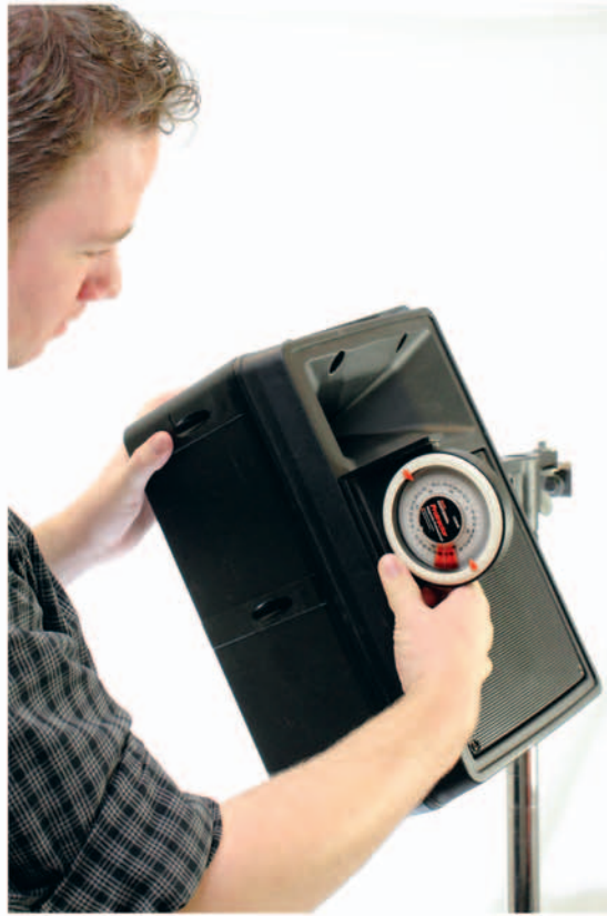
Figure 6.4 Using an Inclinometer to Adjust Speakers
