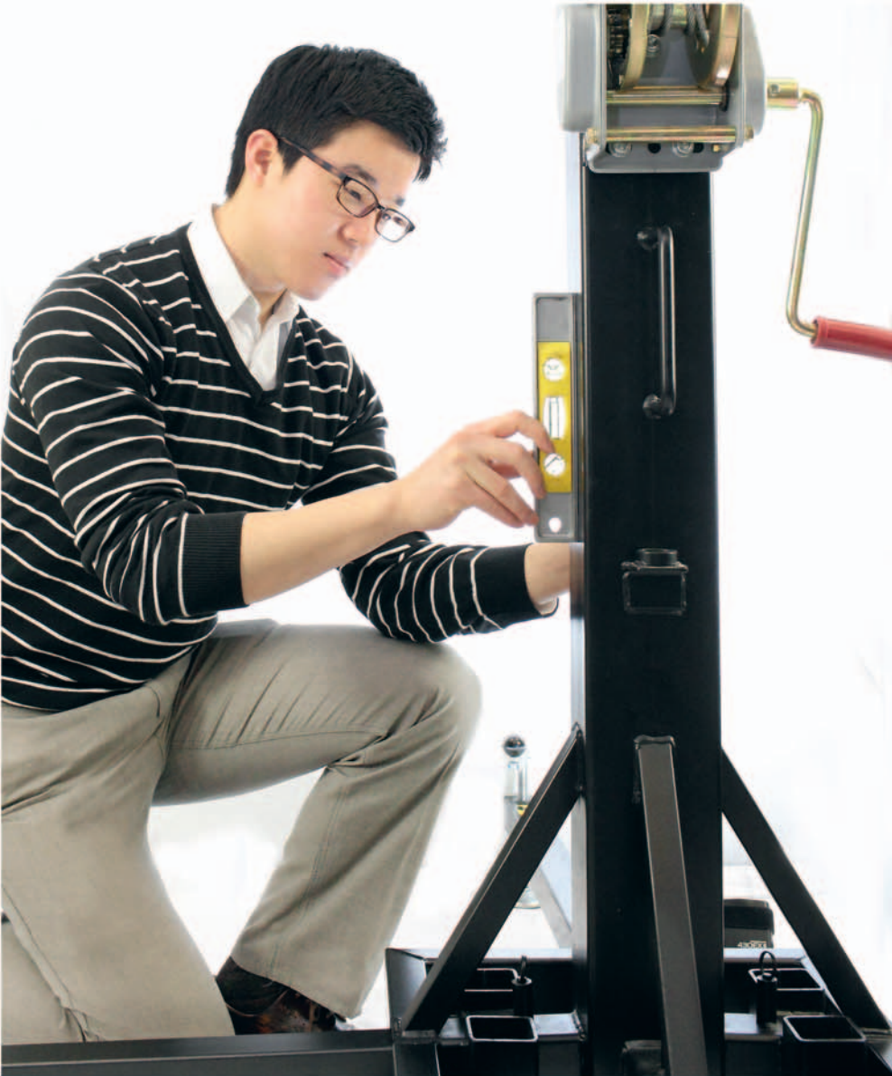
Figure 6.1 Always Verify That Tripods and Towers Are Level
