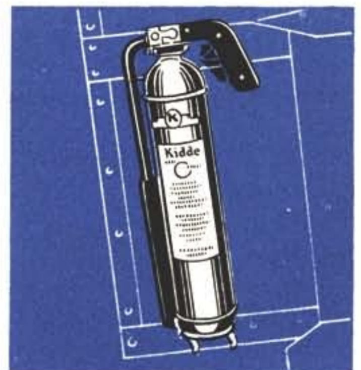
One CO 2 type fire extinguisher is located in the aft pressurized compartment
