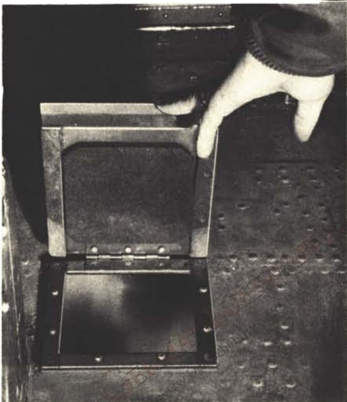
CHECK TO SEE NOSEWHEEL IS STRAIGHT
