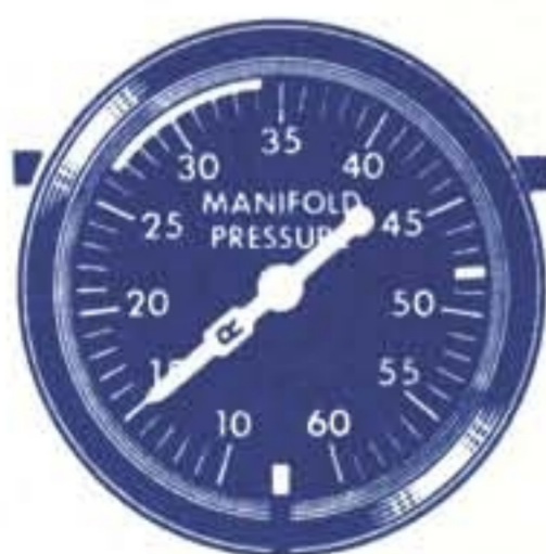
PRACTICE STALLING AT NOT MORE THAN 15" HG.
