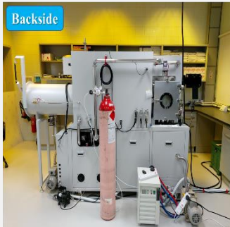
Digitally Controlled Glove Box with Thermal Evaporation System
