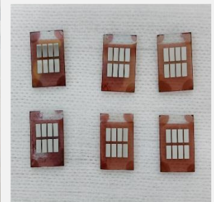
The first solar cell prepared in our lab We used commercial Tin (Sn) metal as a back electrode
