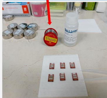
The first solar cell prepared in our lab We used commercial Tin (Sn) metal as a back electrode
