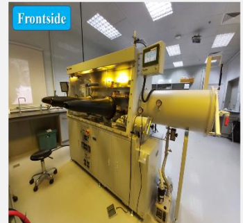
Digitally Controlled Glove Box with Thermal Evaporation System
