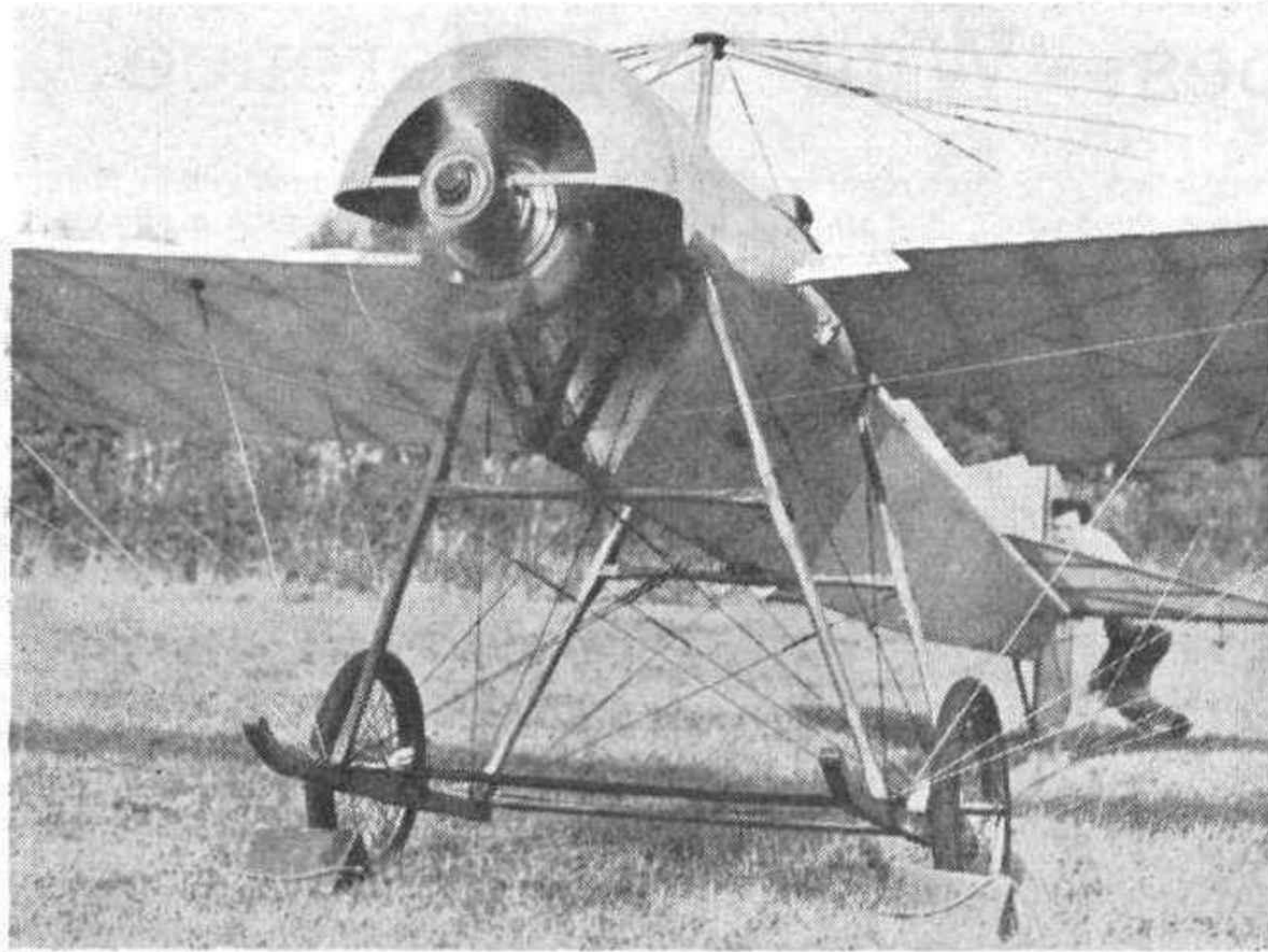
[Photo by "R.A.E. News" Pictures] RUNNING UP the 50-h.p. Gnome rotary engine of the Shuttleworth Trust 1912 Blackburn monoplaner.
