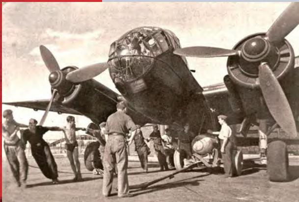
Above German groundcrew load a 1,000kg bomb onto a Ju 188A-2 of I./KG 6. The A-2's engines featured a methanol-water injection system, giving them a different look overall.
